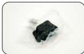
Too much grease
