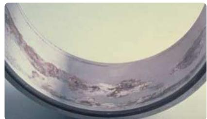
Over time, incorrect contact will result in advanced fretting corrosion. The corroded areas also act as fracture notches (→ figs. 20 and 21).
