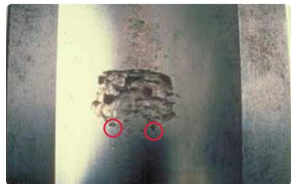
When water, acid or cleaning agents enter an application, it negatively affects the ability of the lubricant to protect steel surfaces from oxidation. As a result, when a machine is at a standstill, deep-seated rust forms easily.
