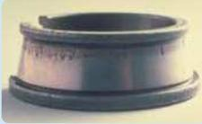
**Rolling surfaces are spalled due to material fatigue**
