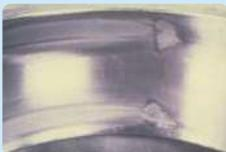
Smearing caused when insufficiently loaded rolling elements slide (skid)
