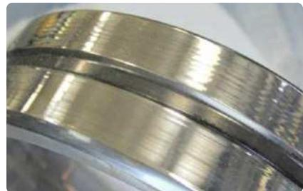
in wear or smearing. The damage is not always confined to the seat surface, but can also have its effect on the side faces of the ring(s). **Fig. 12** shows abrasive wear, while **fig. 13** shows polishing wear.
