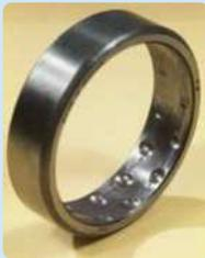
**Rolling surfaces are false-brinelled due to vibration**
