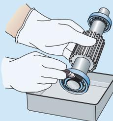
**Solids from manufacturing or previous bearing failures in the housing**
