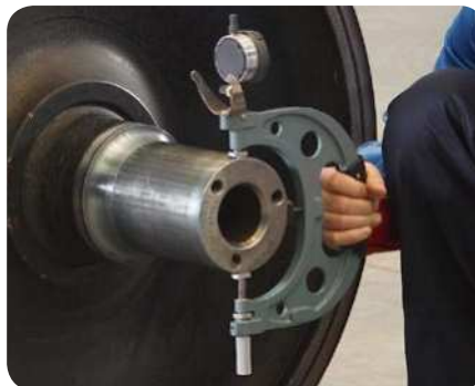
7 Checking the bearing seat diameter, journal end, vertical position
