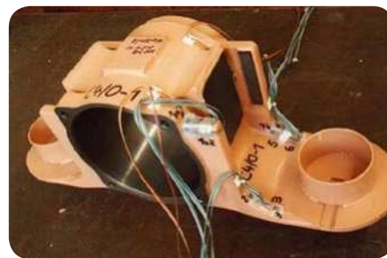
Axlebox equipped with load gauges for validation testing
