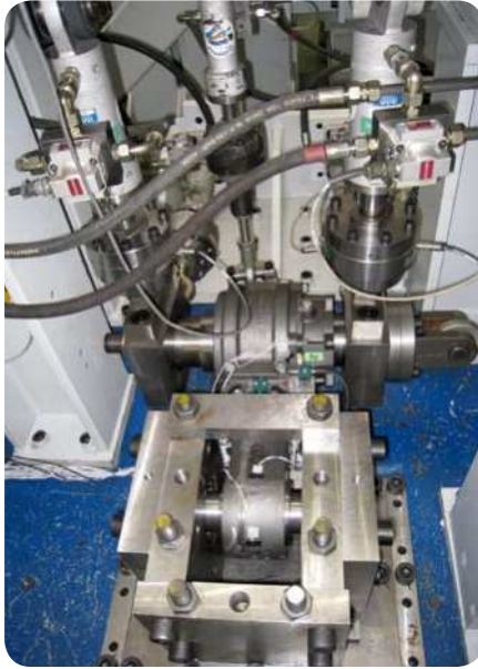
Fatigue testing of a high-speed axlebox housing
