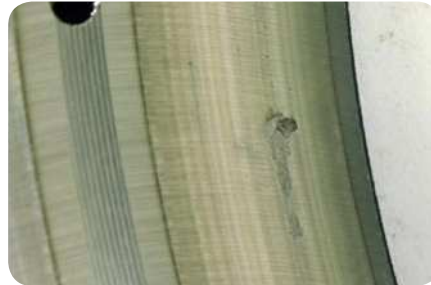
Surface initiated fatigue in the outer ring of a spherical roller bearing. There is surface distress on part of the outer ring raceway. In one place spalling has already started.
