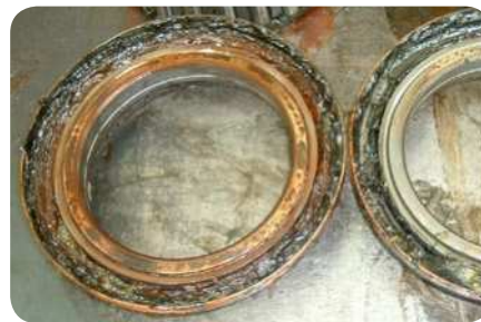
Fretting corrosion on a rear seal and rear inner ring. The grease is discoloured brown due to the fretting debris.
