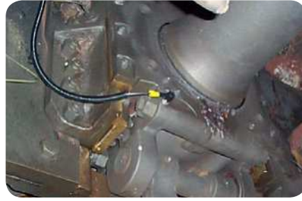
Vibration sensor arrangement in a Swedish MTAB Dm3 locomotive axlebox
