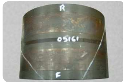
Fretting corrosion marks on the outer ring. The outer ring has a clearance fit in the housing.
