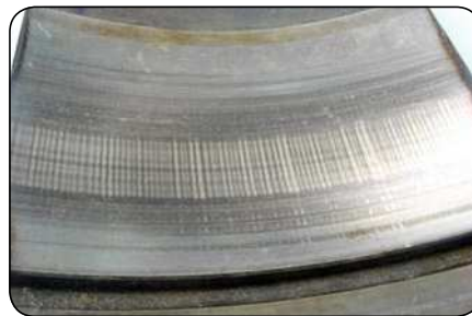
Washboarding in a TBU outer ring The bearing should be scrapped.
