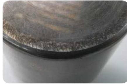
Smearing on the large diameter thrust face of a tapered roller
