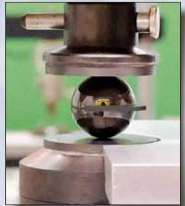
Fig. 5: Principle of the notched ball test for bending strength evaluation of ceramic balls.
