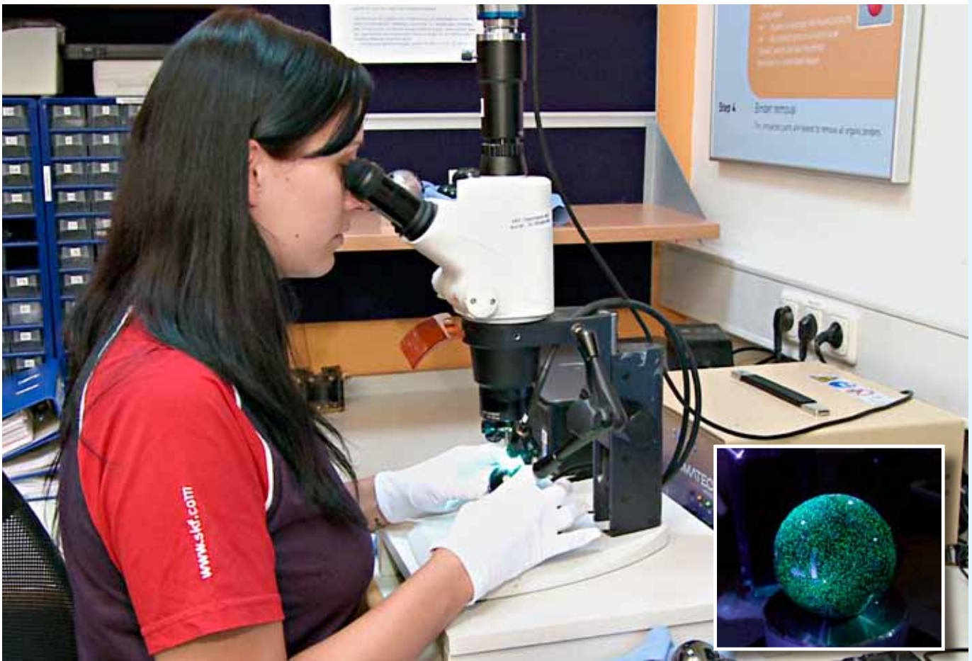
Fig.1: Inspection of 47.625 mm diameter ceramic balls (right) used for windmill generator bearings.
