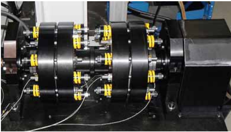
Fig. 9: Endurance life test rig with two sets of four axially loaded 7318 BEMA/HC5DBBVE5752 hybrid angular contact ball bearings.
