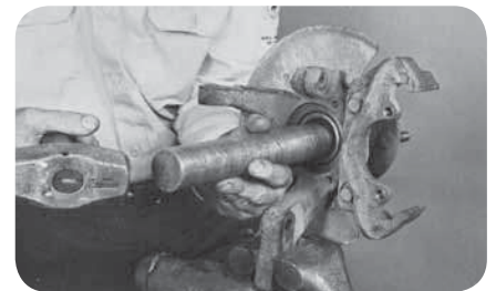
Chrysler – Remove hub from knuckle (fig. 29).
