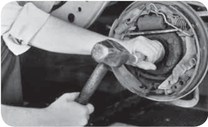
Tap new bearing into shaft cavity (fig. 20).
