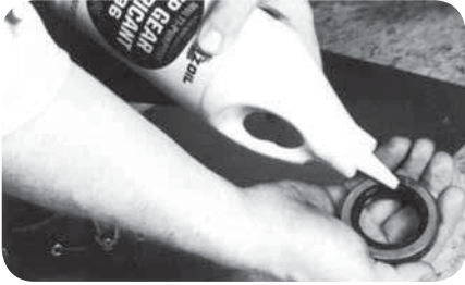
Pre-lube seal with differential lubricant (fig. 19).
