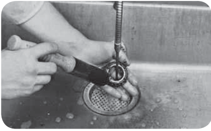
Rinse bearing in clean solvent (fig. 5).
