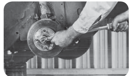
Tighten hub nut while applying brakes (fig. 38).
