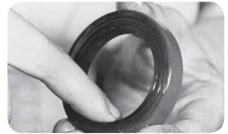
Apply lube to seal lips (fig. 43).
