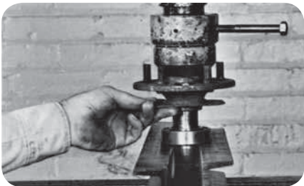
Use arbor press to install bearing (fig. 22).
