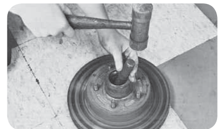
Tap out old seal and inner bearing (fig. 4).
