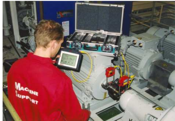
Figure 9. Use of Shims with Laser Alignment Equipment.
