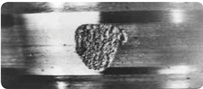
Figure 12. Spalling or flaking on the outer ring of a bearing.
