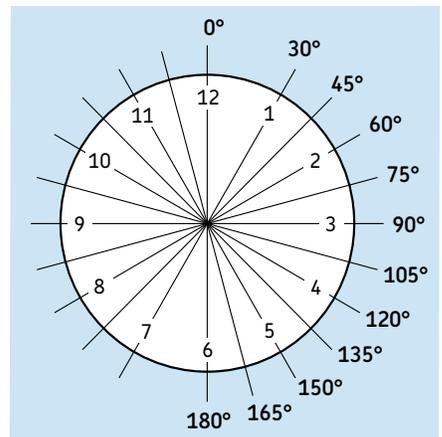
The angles of degree correlate to the hours on a clock. Use this guide to help visualize the turning angles shown on Tables 1 and 2.
