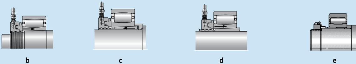
\* Values given valid for HMV (C) E series hydraulic nuts equal to bearing size and with one sliding surface (see Figures b and c). Surfaces lightly oiled with light oil.
