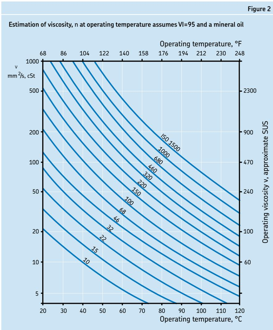
The viscosity obtained from **Figure 1** or from the “rules of thumb” is the viscosity required at the **bearing operating temperature**. Since viscosity is temperature dependent, it is necessary to reference temperature when referring to viscosity.
