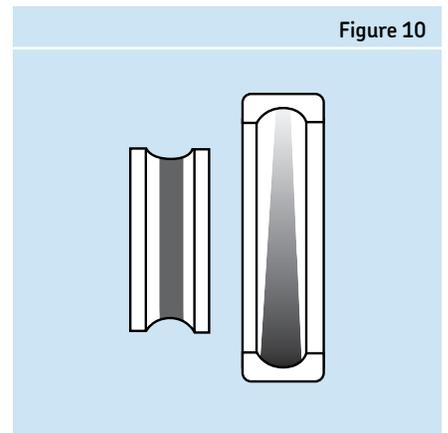
*Load zones produced by out-of-round housing pinching outer ring*
