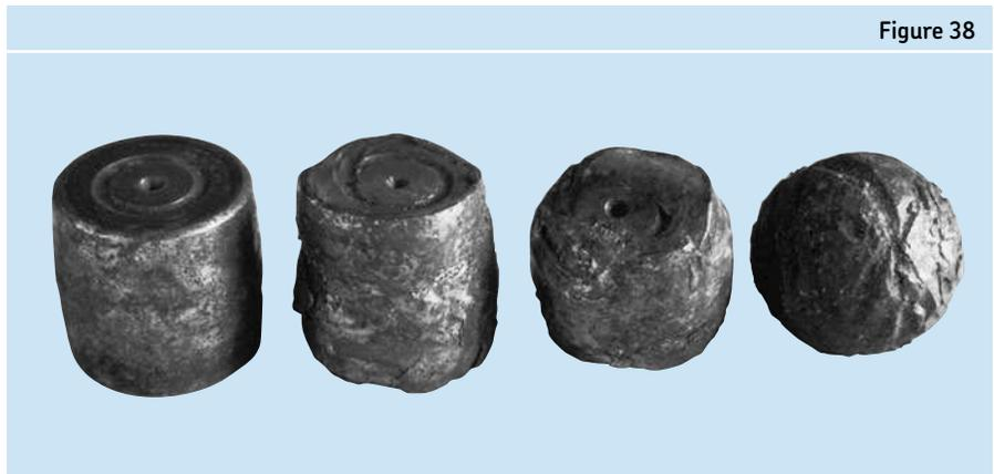
Progressive stages of spalling caused by inadequate lubrication
