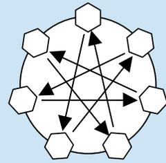
Tightening pattern for set screws
