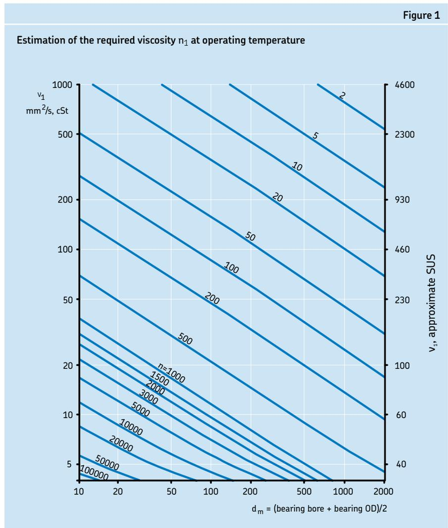
millimeters, where  $d_m = (\text{bearing bore} + \text{bearing OD})/2$ . Speed, in rpm, is given on the diagonal lines. To determine the minimum required viscosity at the bearing operating temperature, find the point where the mean diameter and speed lines intersect – then read across horizontally to the vertical axis on the left to determine the minimum required viscosity in centistokes, or to the right to determine the minimum required viscosity on Saybolt Universal Seconds.
