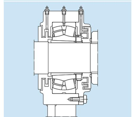
relubrication per time unit is derived from the equations for  $G_p$  under "Replenishment" by spreading the relevant quantity over the relubrication interval. When using continuous relubrication, check whether the grease can be adequately pumped if ambient temperatures are low. Continuous lubrication can be achieved via single-point or multi-point automatic lubricators, e.g. SKF SYSTEM 24<sup>®</sup> or SYSTEM MultiPoint.
