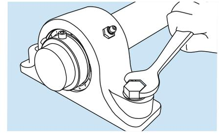
When the inboard locking collar is inaccessible and cannot be tightened like in the case of a F6BRPE piloted flange with a blind hole installation, the unused inboard locking collar should be removed from the bearing inner ring before installation. This avoids an unused component coming loose during operation.
