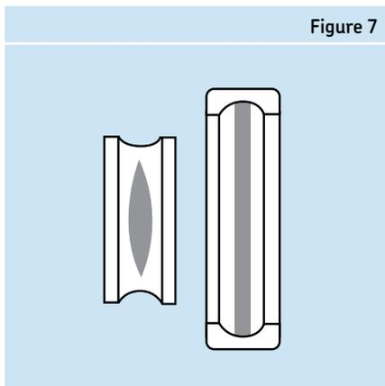
Load zone when thrust loads are excessive
