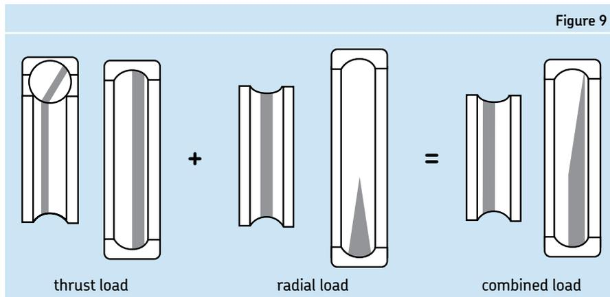
*Load zone from internally preloaded bearing supporting radial load*
