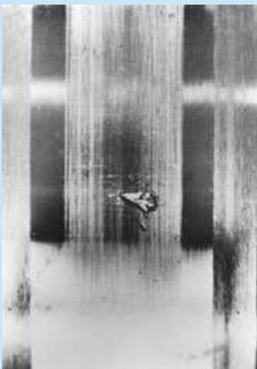
Early fatigue spalling
