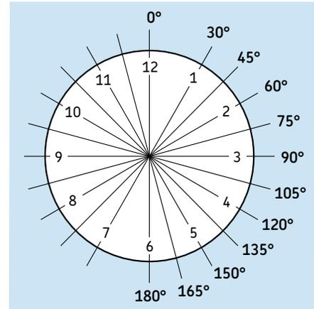
The angles of degree correlate to the hours on a clock. Use this guide to help visualize the turning angles shown on Table 4.
