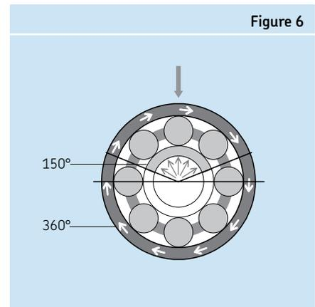
Normal load zone outer ring rotating relative to load or load rotating in phase with inner ring
