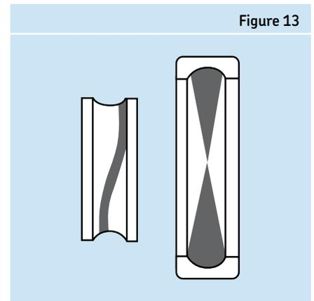
**Figure 13** illustrates the load zone produced when the inner ring is misaligned relative to the shaft axis. This condition can occur when the shaft is bent and generates what is referred to as a dynamic misalignment condition.
