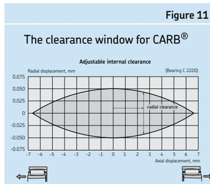
For example, if the axial displacement is 2.5 mm, the radial clearance is reduced from 100 to 90  $\mu\text{m}$  and the radial position of the bearing changes from  $-50$  to  $-45$   $\mu\text{m}$ , (**Figure 11**). For more information please contact SKF.
