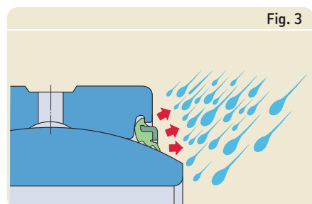
Three seal lips keep contaminants out
