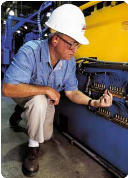
A maintenance technician is adjusting injector output to one bearing on a roll forming machine. More than 100 points are being lubricated from one pump without shutting down the machine.
