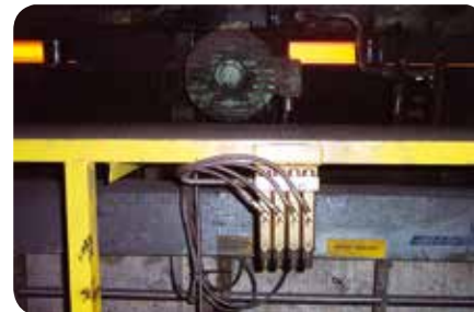
These SL-V injectors operate in a harsh steel mill environment that includes high heat and abrasive contamination. Purging the bearings, replacing the grease film frequently and increased safety are key benefits of this system.
