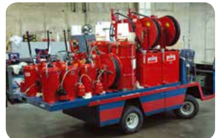
In-plant lubrication trucks take all the important fluid lubricants to the machinery. This electric cart even includes a waste oil evacuation system.
