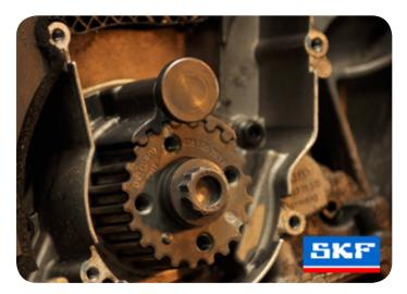
4. Lock camshaft sprocket and crankshaft sprocket using the correct tools.
