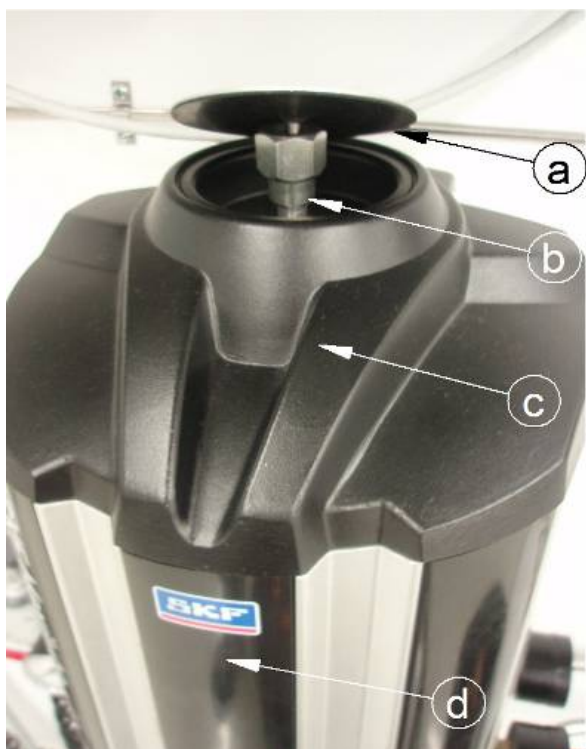
Figure 16 Accessing the inner parts of the pumping center
