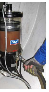
Turbines require large volumes of grease to be dispensed during each lubrication maintenance session. Even though SKF WindLub lubrication systems require minimal maintenance, lubricant must be refilled from time to time. Tower heights and tight working spaces create unique challenges for maintenance workers.
