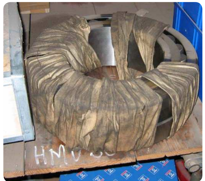
Fig. 5 Bearing stored without protection from dust.
