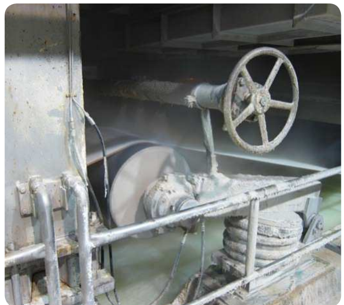
Fig. 7 The high humidity environment of a wire stretch roll in a paper machine forming section. Grease in the labyrinth seal stops process water entering the bearing housing.
