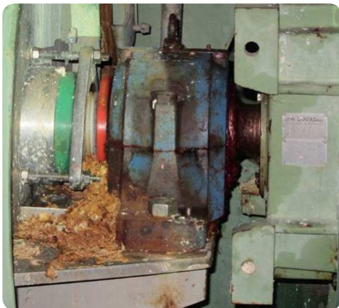
Fig. 6 Fibre leaking out of the gland seal on a pulp washer. Note the additional protection in front of the housing to protect the housing seal.
