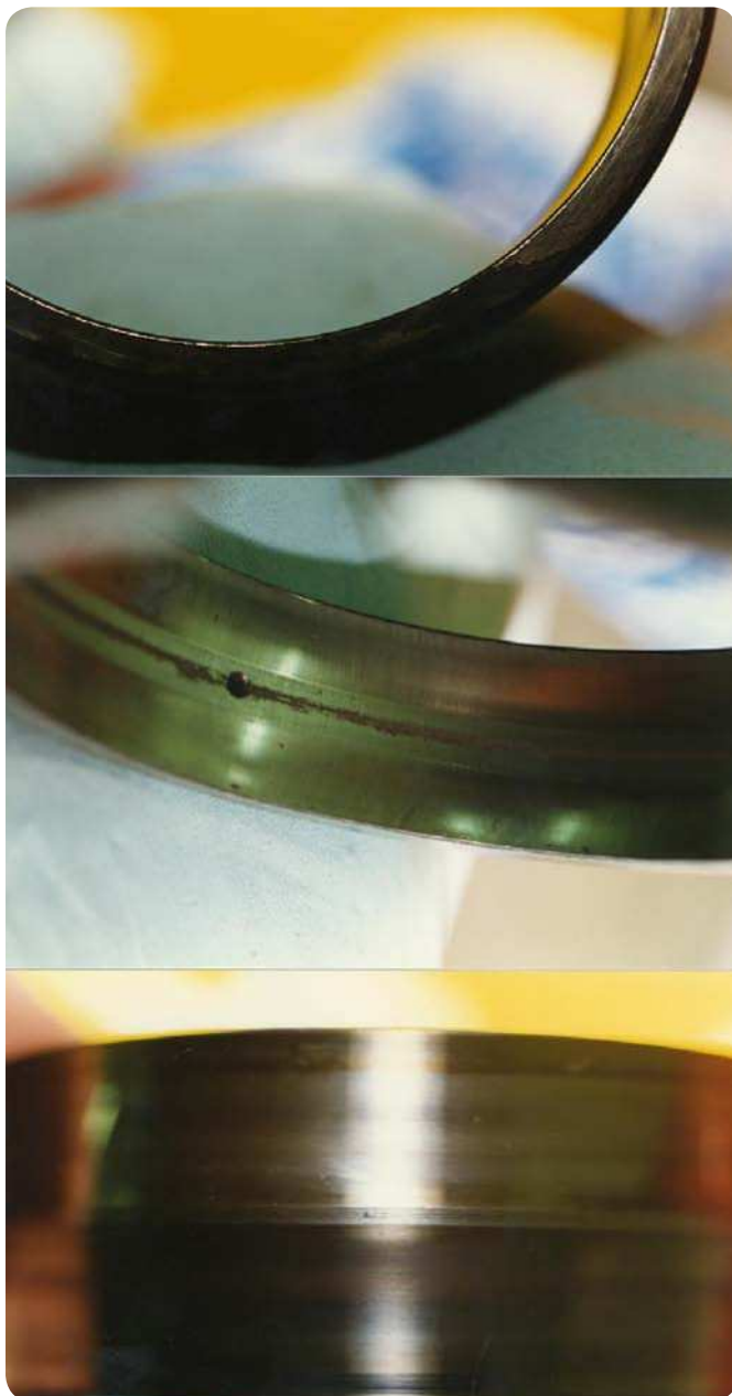
Fig. 13 Solid Oil bearing after 8 months in operation on a felt roll with water in the housing. The water level in the housing can be seen from the corrosion on the outer ring side face in the upper photograph.
