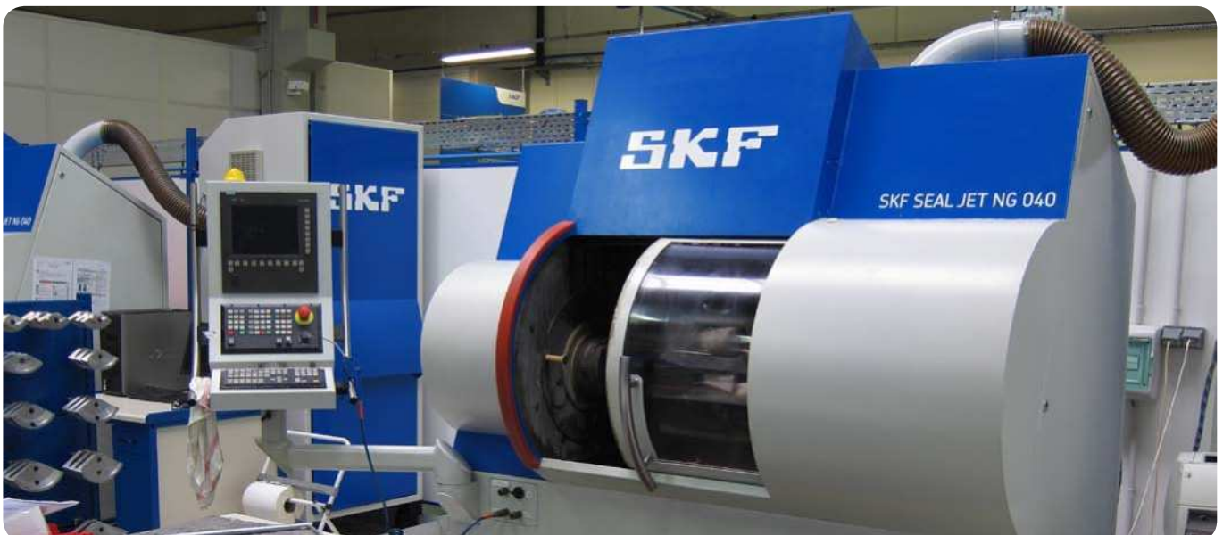
Fig. 10 SKF SEAL JET is able to machine polymeric seals to tailor made shapes and dimensions to fit a customer's application. It is often used as an alternative in cases where adding a standard seal to increase sealing efficiency requires costly modifications.
