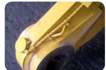
High impact areas where most of the grease is used and system is heavily guarded
