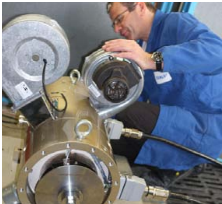
Fig. 3: 75 kW PM motor – final check before shipping.
