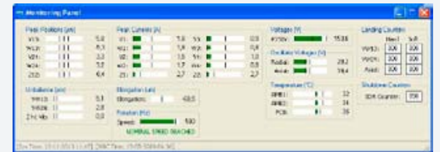
Fig. 4: Screenshot of MBScope software taken during field operation. One can monitor most of the operating parameters: rotational speed (here, the motor is operating at 35,000 r/min), vibration level per axis (less than 6 microns), vibration due to imbalance, shaft elongation, temperature, current and voltage.
