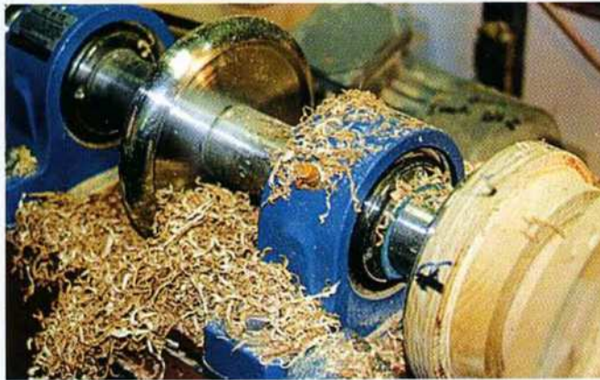
The Pop Release bearing unit mounted in a wood working lathe (Photo 1).
