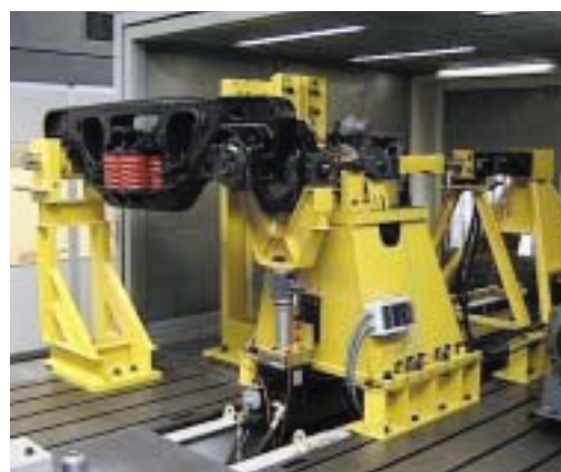
The THISBE test rig simulates real operating conditions that are recorded in service.
