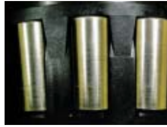
Compact TBU class G after 570,000 km heavy-haul freight service. From left to right: CTBU before dismantling; outer ring (cup) raceway; polymer cage and rollers.
