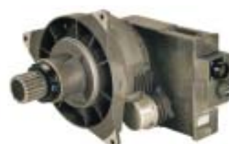
The door actuator developed for the Dassault Falcon 2000.
