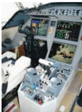
Fly-by-wire functions can include the interface between the pilot and the flight control computers.
