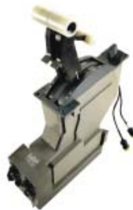
The throttle control unit transmits the pilot's control movements to the engine.
