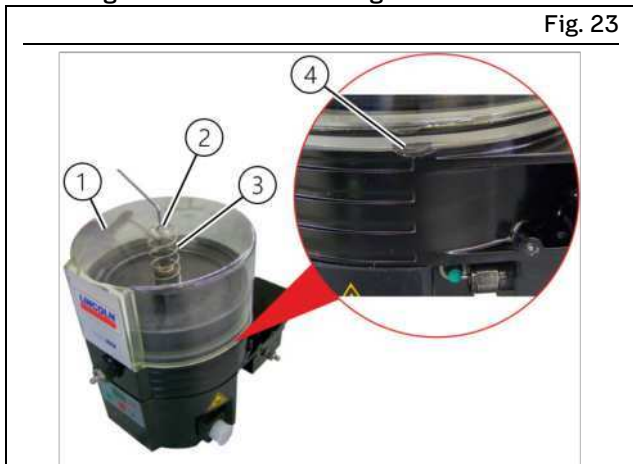
Unfastening and removing the reservoir
