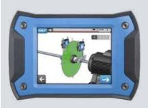
Free measurement allows alignment measurements to start at any angle and finish with an angular sweep of just 90°.
