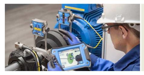
Shaft alignment is recommended for almost every industry, as it enables machine uptime to be significantly improved and maintenance costs to be reduced. The simplicity of the TKSA 41 provides greater confidence for the performance of alignment tasks on all types of horizontal rotating machines.
