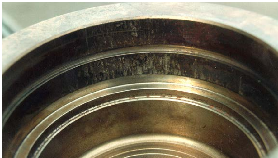
Fig. 7 Fretting corrosion in the housing
