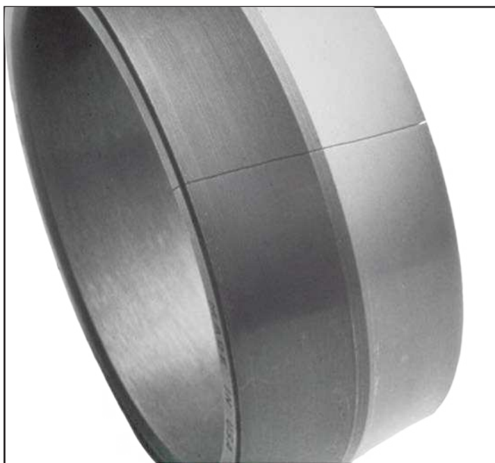
Fig. 16 The fractured inner ring of a spherical roller bearing resulting from excessive drive-up
