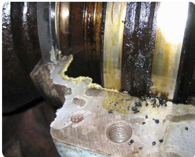
Fig. 7 Oil transformed into carbon.
