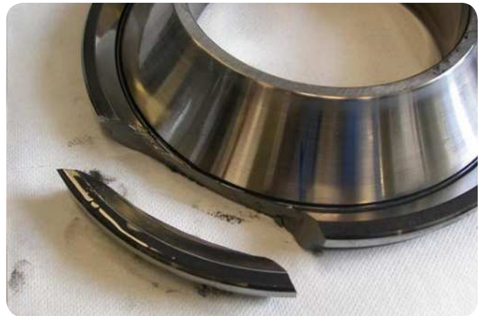
Fig. 1 Bearing with cracked shaft washer
