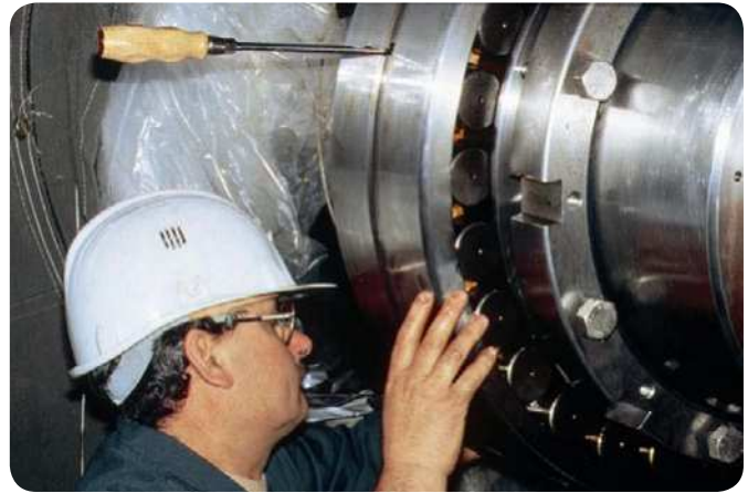
Fig. 7. Rotating the outer ring with a clean screwdriver.
