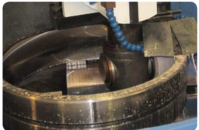
Fig. 10 Level 4 grinding of a spherical roller bearing outer ring
