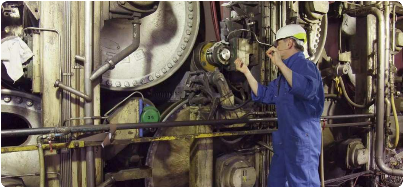
Philippe Gachet using a wire tool to check the condition of the raceway on a felt roll bearing.
