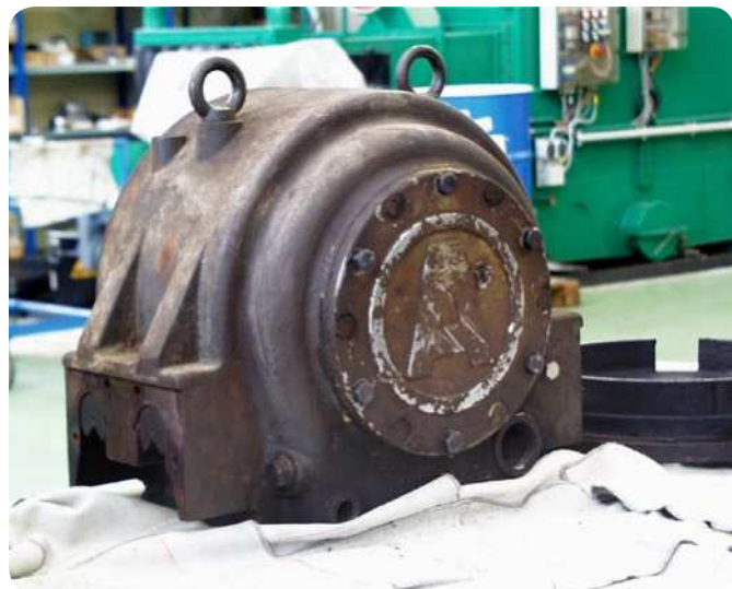
Fig. 13 Rocker housing before modification.
