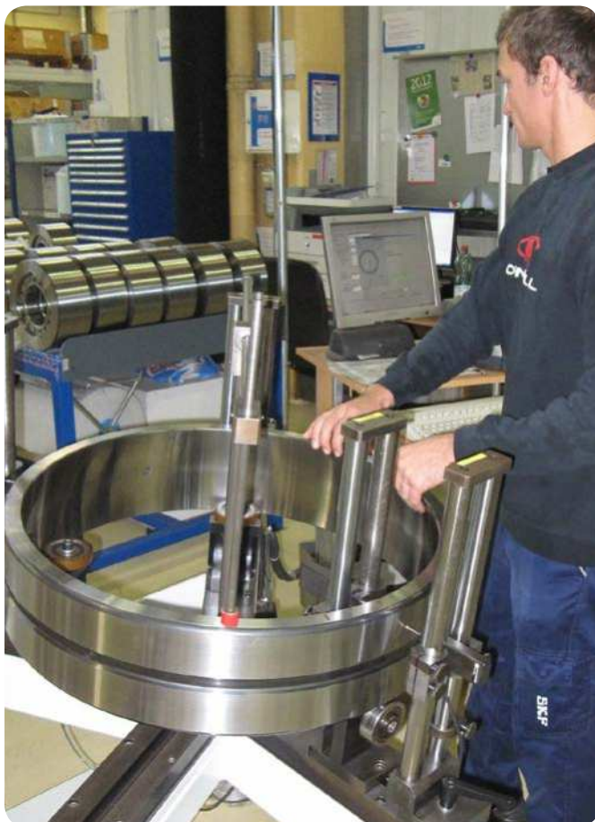
Fig. 11 Ring ovality and wall thickness variation measurement
