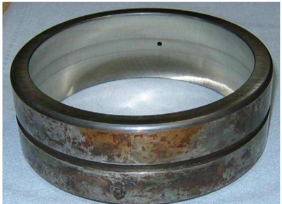
Fig. 1 Fretting corrosion on the outer diameter of a spherical roller bearing
