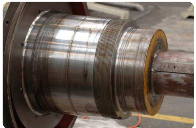
Fig. 7 Strange contact pattern on a journal.
