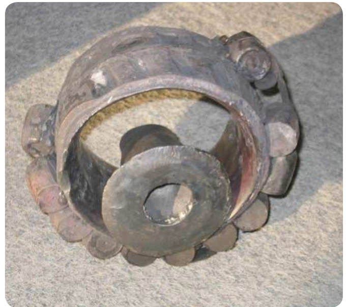
Fig. 2 A bearing that is too badly damaged to diagnose the probable failure cause. The part in the middle is what remains of the shaft that supported the bearing.
