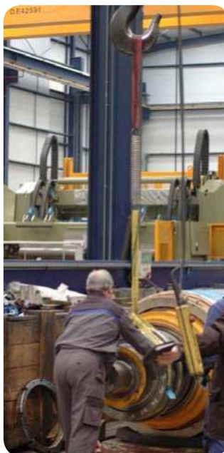
Fig. 5 Using a spring to make mounting heavy bearings easier.
