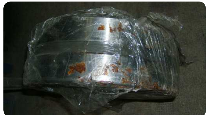
Fig. 3 Bearing, in storage, corroded by humidity.
