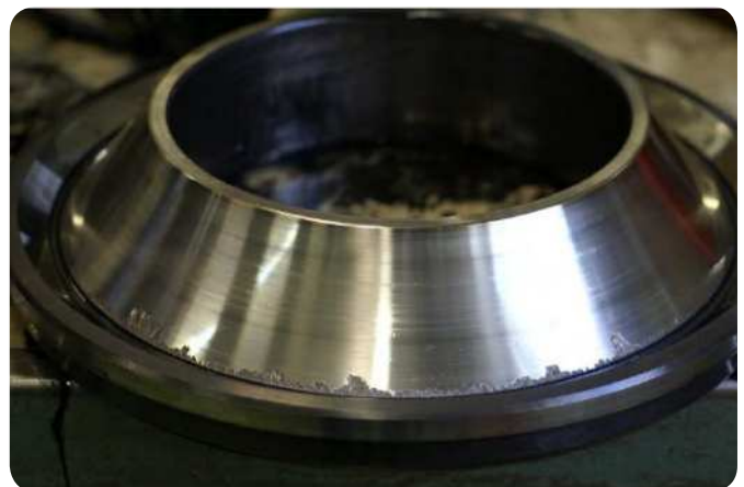
Fig. 2 Bearing made from upgraded steel with spalling
