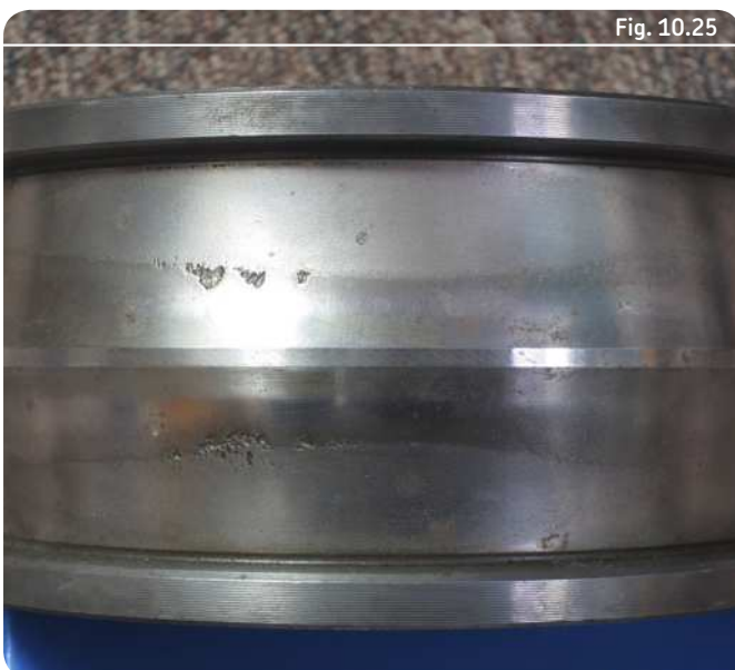
Surface distress on a felt roll bearing contaminated with process water
