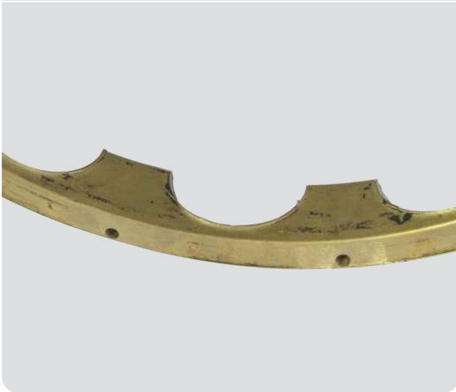
Deep groove ball bearing cage with burrs due to abrasive wear due to a too long relubrication interval
