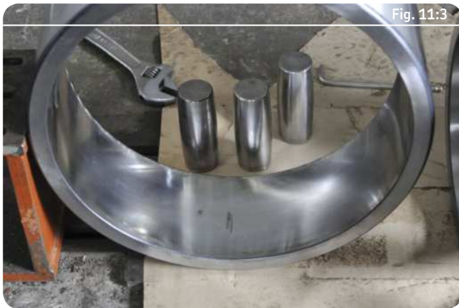
Light surface standstill corrosion on a CARB toroidal roller bearing
