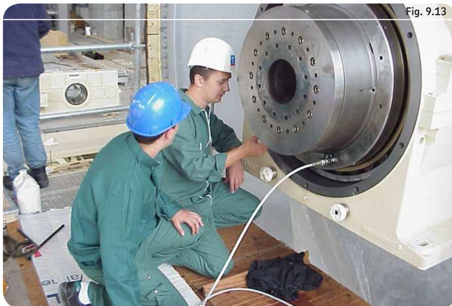
Mounting a CARB toroidal roller bearing on a Yankee cylinder using the SKF Drive-up Method
