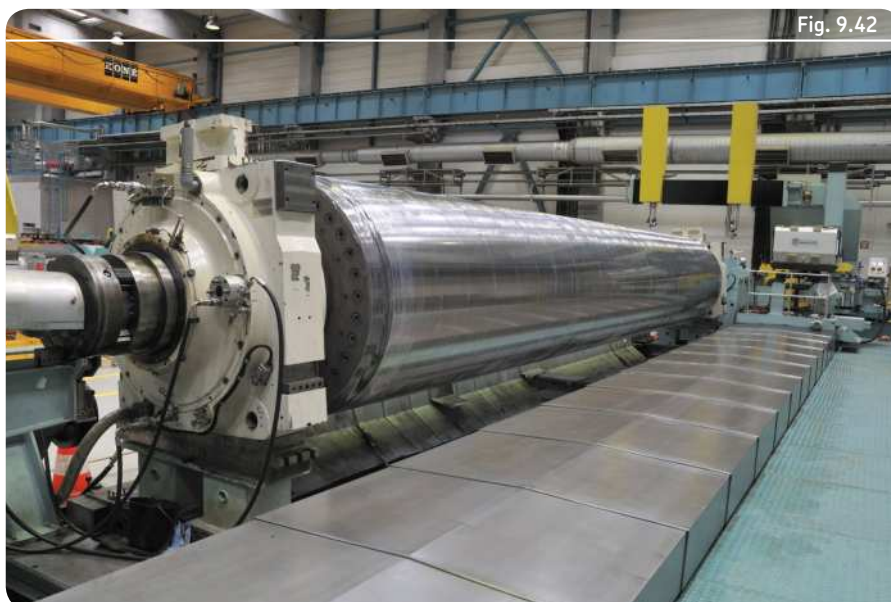
Thermo roll being reground and rotated on its main bearings
