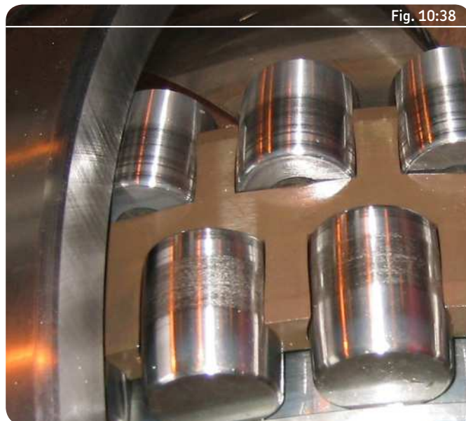
Micro smearing marks on the rollers of a deflection-compensating press roll
