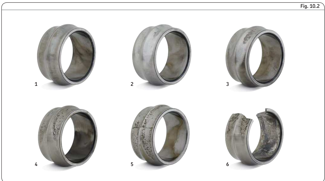
The development of bearing damage
