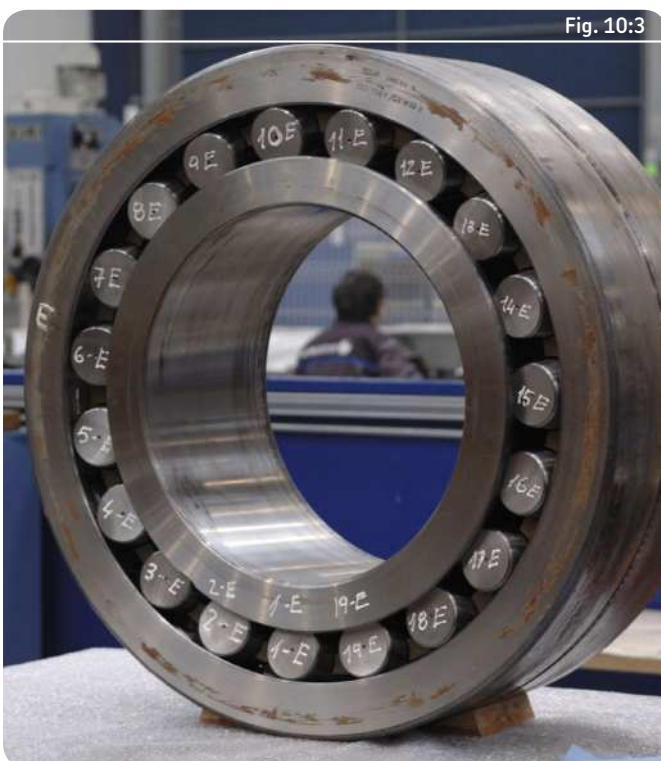
Press roll bearing rings and rollers marked with "E" for the external side
