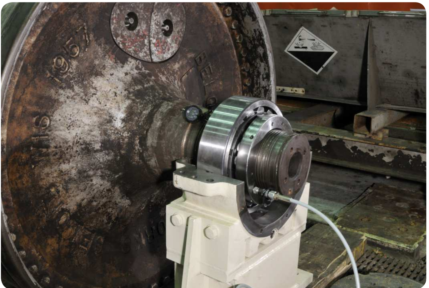
CARB toroidal bearing mounted on an old drying cylinder as an upgrade
