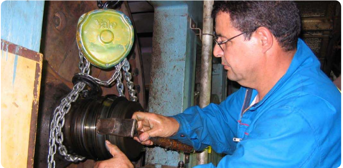
SKF technician checking bearing seat geometry with an inner ring and Prussian blue
