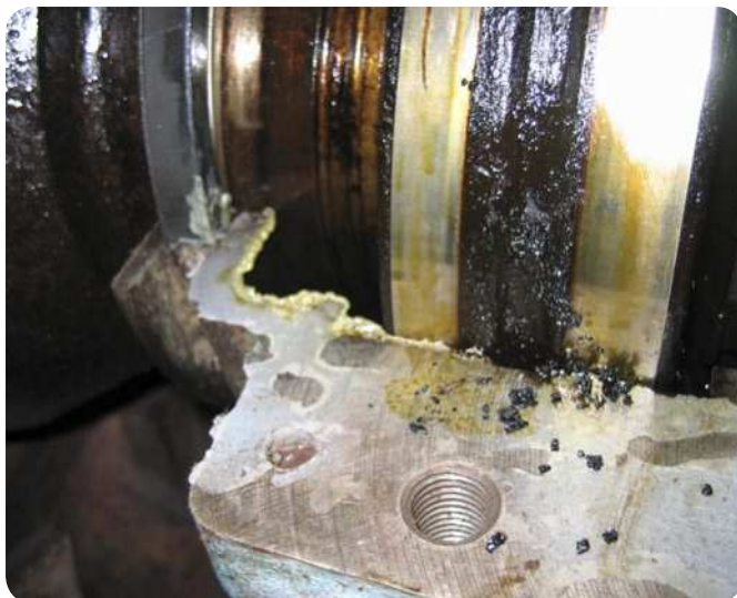
Fig. 7 Oil transformed into carbon.
