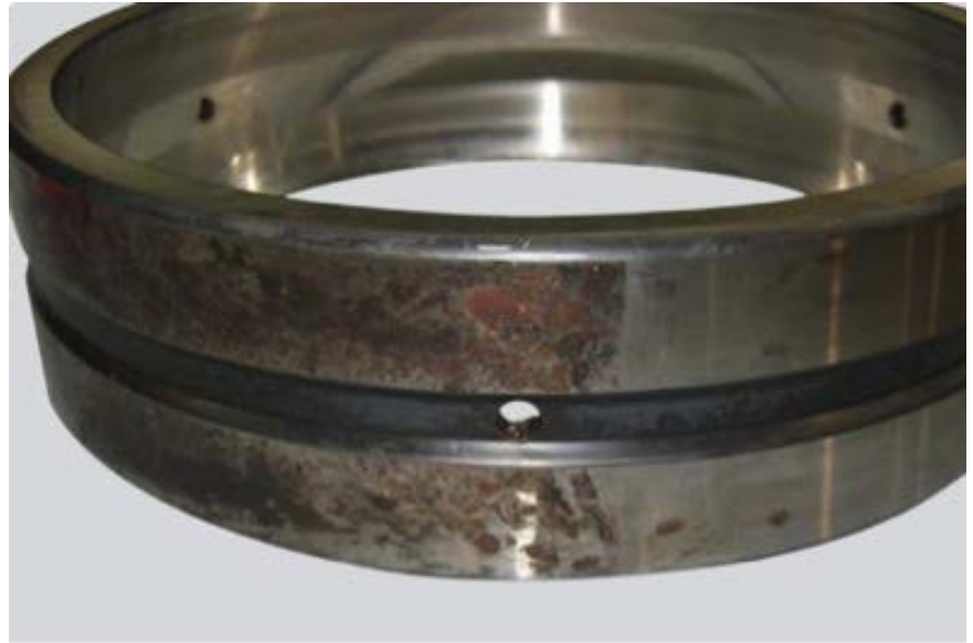
Fig. 18 Oval clamping due to mismatched cap and base on a split plummer block housing
