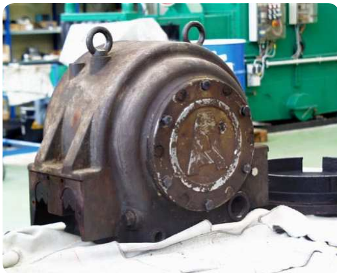
Fig. 13 Rocker housing before modification.
