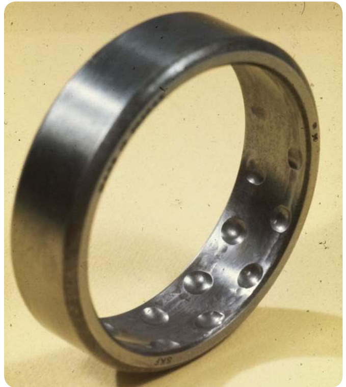
Fig. 4 An outer ring of a self-aligning ball bearing that has been subjected to false brinelling.
