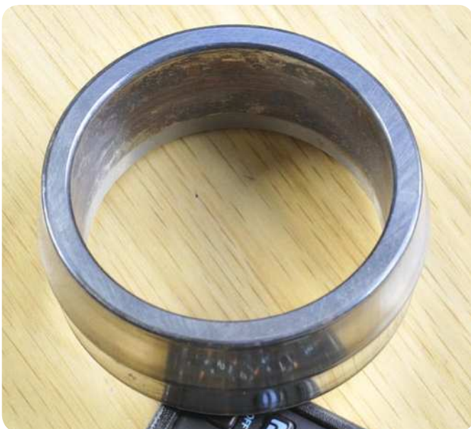
Fig. 1. Inner ring of a spherical roller bearing showing fretting corrosion in the bore because of an insufficiently tight fit.
