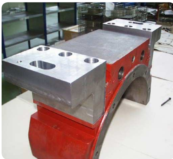
Fig. 5 The housing base is machined to remove the rockers and to accept customized feet. The oil inlet and outlet are also modified.
