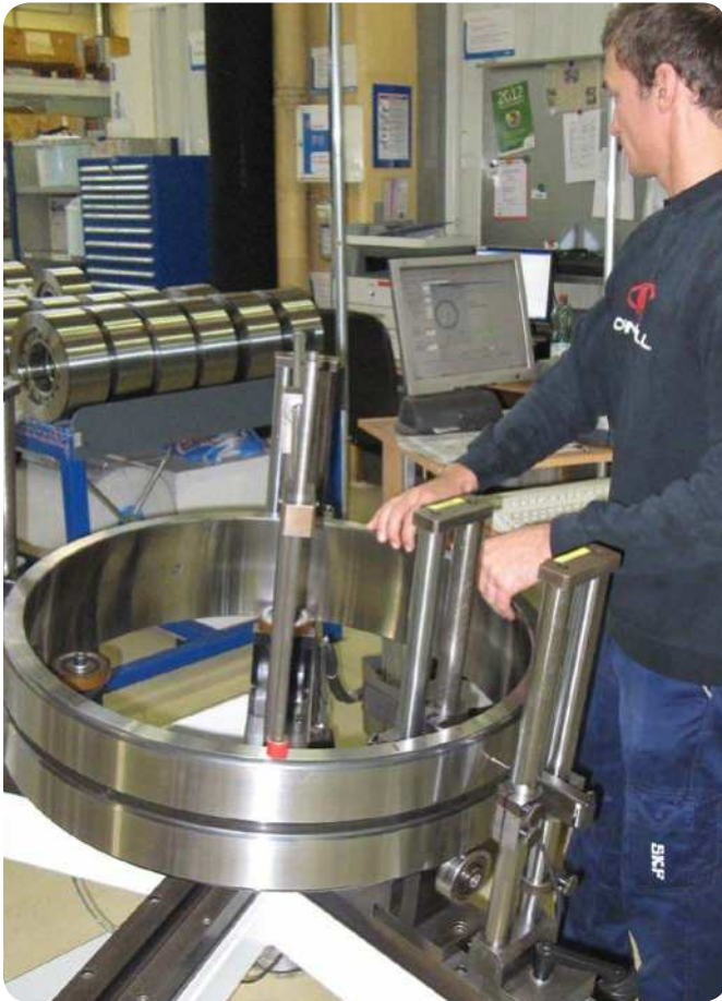
Fig. 11 Ring ovality and wall thickness variation measurement
