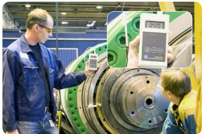
Fig. 4 The handheld device shows 0,420 and the Metso's technician gets ready to switch off the air drive oil pump connected to the HMV hydraulic nut.
