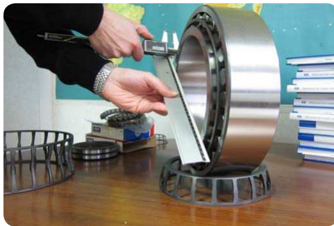
Fig. 7 Using a ruler and a vernier caliper to measure inner ring versus outer ring axial offset I.
