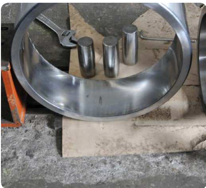
Fig. 8 Dismounted CARB toroidal roller bearing at a paper mill ready for inspection before being sent for remanufacturing
