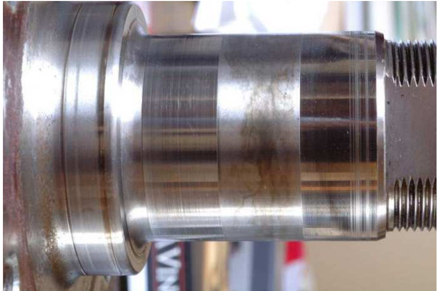
Fig. 4 Wheel bearing stub axle showing wear in the contact surface with the tapered roller bearings due to a loose fit and changing load direction after 200 000 km
