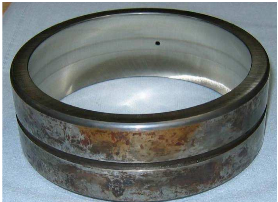
Fig. 1 Fretting corrosion on the outer diameter of a spherical roller bearing
