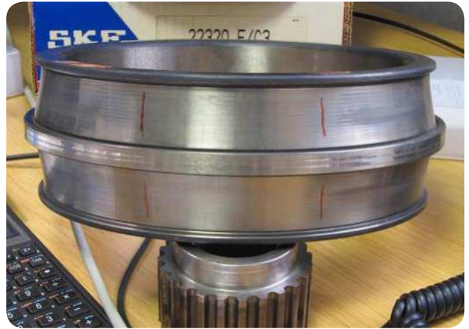
Fig. 3 The inner ring of a drying cylinder bearing with no load zone between the red lines.
