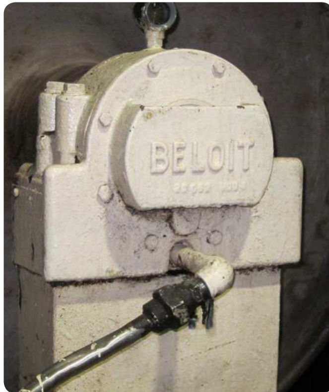
Fig. 4 A rocker housing on an old paper machine.
