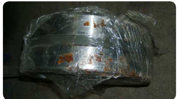
Fig. 3 Bearing, in storage, corroded by humidity.
