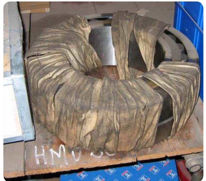
Fig. 5 Bearing stored without protection from dust.
