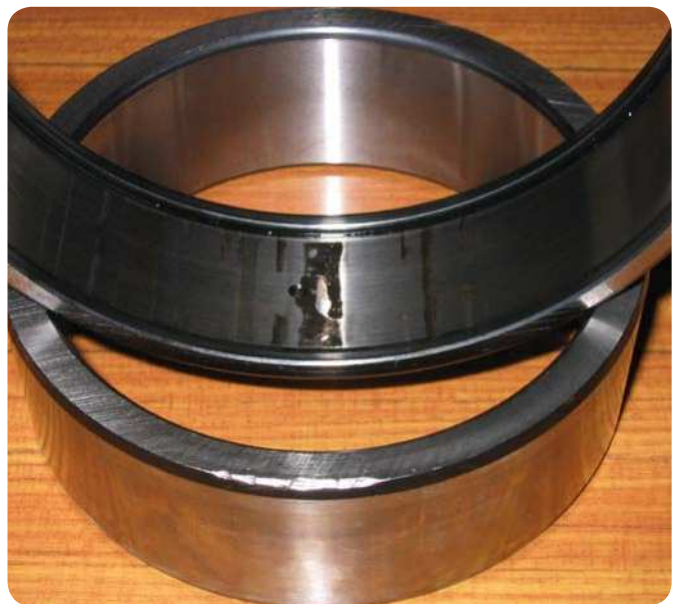
Fig. 2 Standstill corrosion in a needle roller bearing from a tissue converting plant. The machine it was mounted on had been cleaned with high pressure water.
