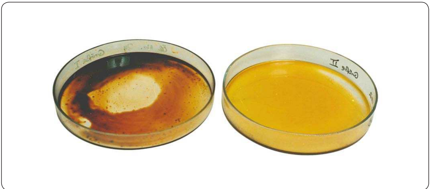
Fig. 8 SKF oil ageing test. On the left is synthetic oil after four weeks at 140 °C (284 °F), it has lacquered and the evaporation loss is 93%. On the right is a mineral oil after 4 weeks at 120 °C (248 °F) with an evaporation loss of only 2%.
