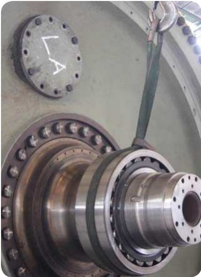
Faulty Prussian blue test due to too low axial force on the bearing
