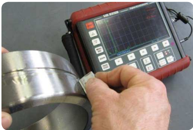
Fig. 3 Ultrasonic testing for subsurface micro cracks in the outer ring of a spherical roller bearing.
