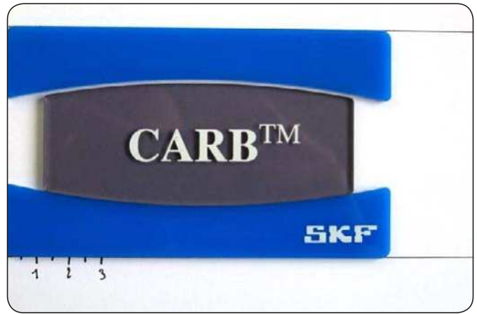
Fig. 4 Inner and outer rings aligned, roller in the equilibrium position and limited radial clearance. Note the scale is in cm.
