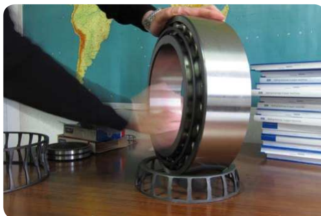
Fig. 9 Rotating the inner ring to free up a bearing blocked by too much axial displacement.
