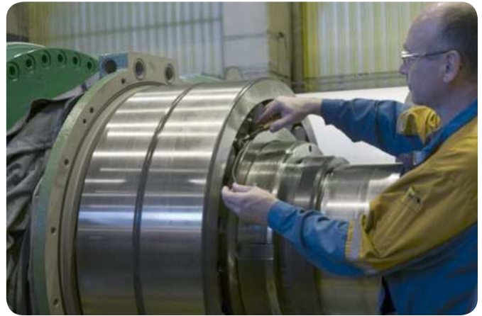
Fig. 7 A Metso technician cuts off the sensor cable.
