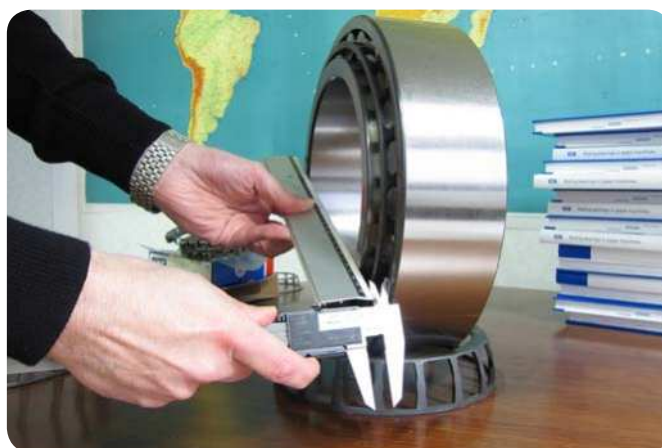
Fig. 8 Using a ruler and a vernier caliper to measure inner ring versus outer ring axial offset II.
