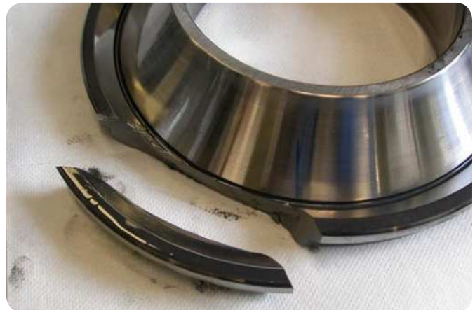
Fig. 1 Bearing with cracked shaft washer
