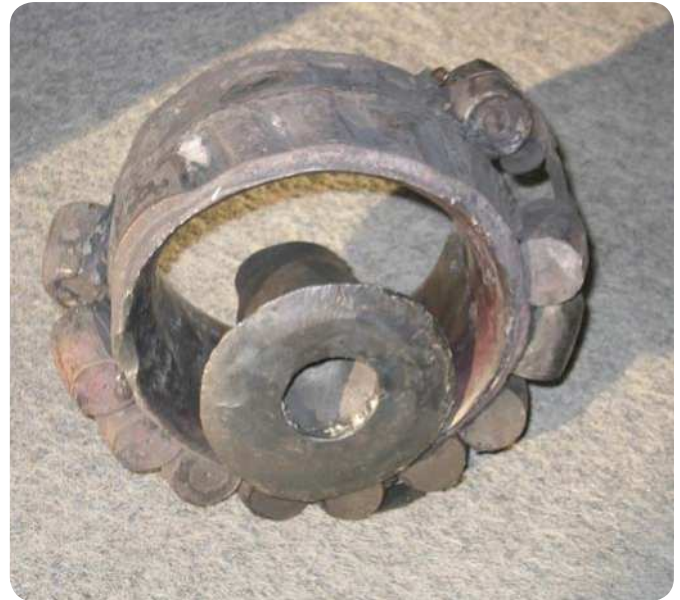
Fig. 2 A bearing that is too badly damaged to diagnose the probable failure cause. The part in the middle is what remains of the shaft that supported the bearing.
