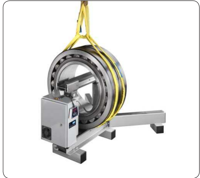
Fig. 1 SKF TIH L induction heater for bearings up to 800 mm bore diameter and 1 200 kg weight e.g. many Yankee cylinder bearings.
