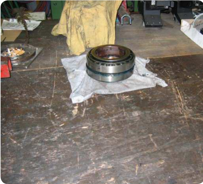
Fig. 2 Wooden workbenches are difficult to clean properly.
