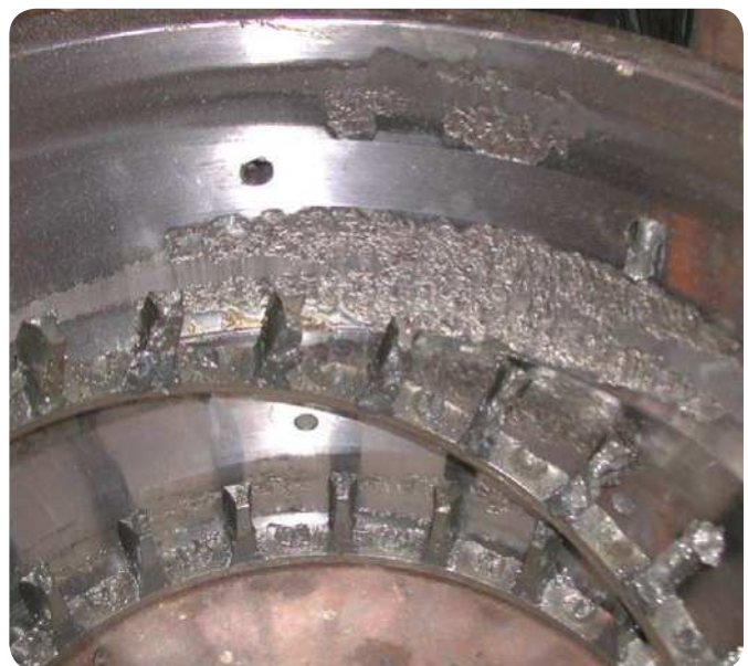
Fig. 1 Surface distress and spalling can be seen on the outer ring raceway of this wet section press roll bearing. The cause is inadequate lubrication. The remaining grease on the cage looks like it has been contaminated with water which leads to the conclusion that inadequate lubrication is the consequence of liquid contamination. If no grease was present, it is likely that the failure analysis would have incorrectly been simply inadequate lubrication.
