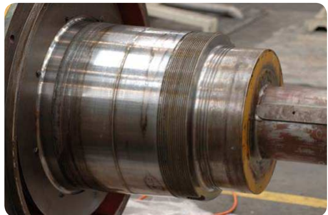
Fig. 7 Strange contact pattern on a journal.
