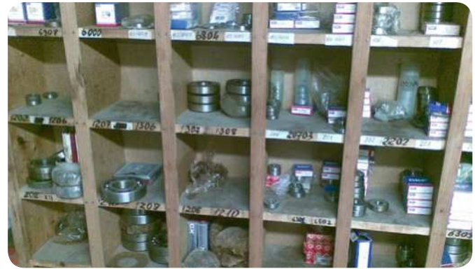
Fig. 1 Bearings, if left unpackaged, collect dust
