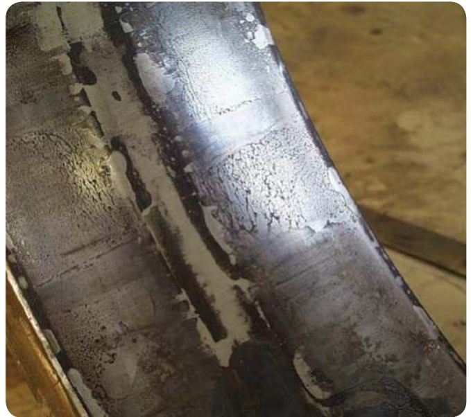
Fig. 3 The outer ring of a spherical roller bearing that was mounted on a paper machine.
