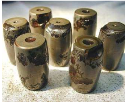
Rollers from a counterfeit spherical roller bearing
