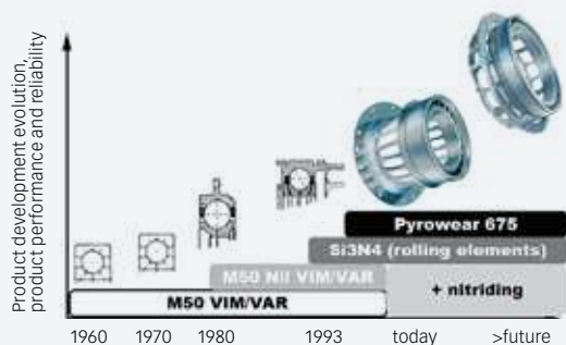
Fig. 7: Advances in materials, thermal processing and manufacturing technology have all been key enablers in the evolution of main-shaft engine bearings, including both increased performance and ability to include integrated structures.
