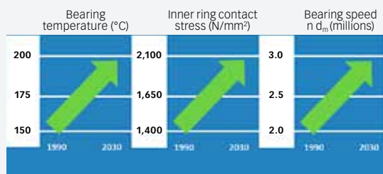
Fig. 8: Aerospace main-shaft engine ball bearing (thrust load) peak operating condition trends enabled by material, design and manufacturing advances.
