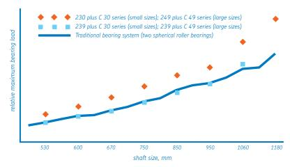
The SKF total trunnion solution provides three options depending on customer need.
