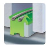
The SKF total trunnion solution includes a new acrylonitrile-butadiene rubber (NBR) seal. The seal, which can accommodate 1,5° of misalignment, incorporates a metal ring to protect against hot dust and slag. This new seal can accommodate temperatures up to 100 °C (212 °F).
