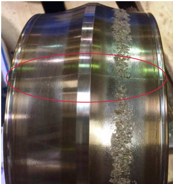
Fig. 16: Damaged bearing inner and outer rings
