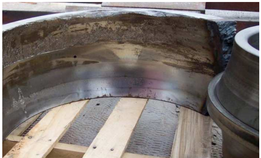
Fig. 7: Severely damaged bearing outer race
