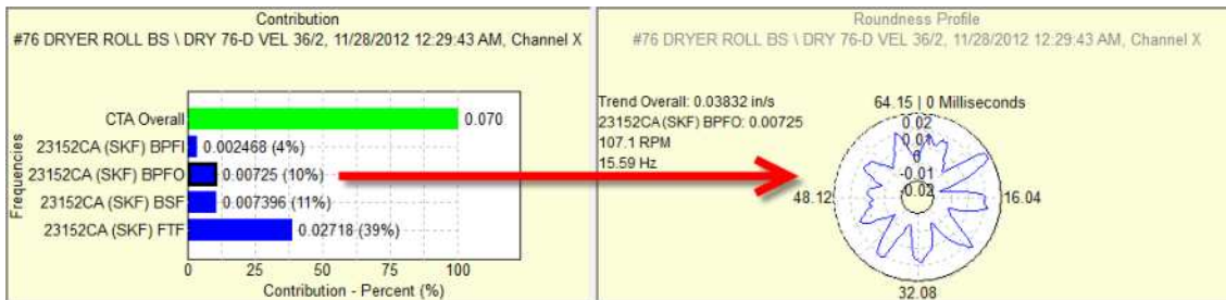
Figure 2 - 5. The Roundness Profile Plot with a Frequency Bar Selected.
