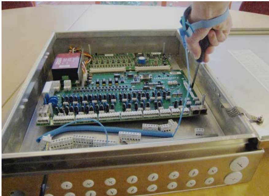
Figure 4 - 7. Always Use an ESD Wrist Strap When Handling the Lightning Protection Board.
