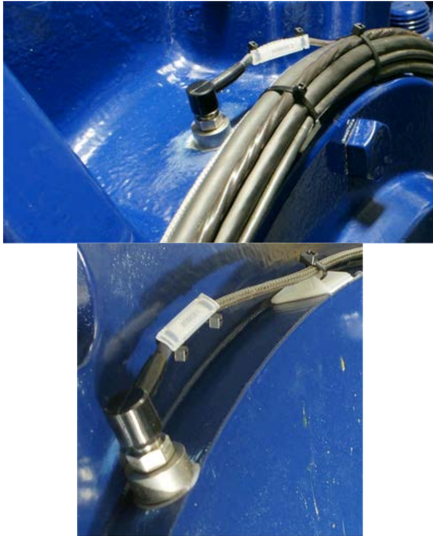
Figure 3 - 3. Examples of Attachment by Glue.
