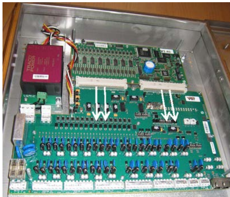
Figure 4 - 9. Pull the Lightning Protection Board down to Free It from the CPU Board.
