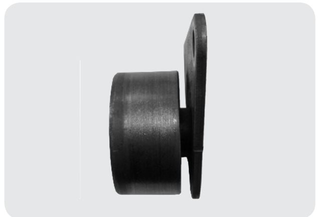
Pulley misalignment caused by bent back plate.
