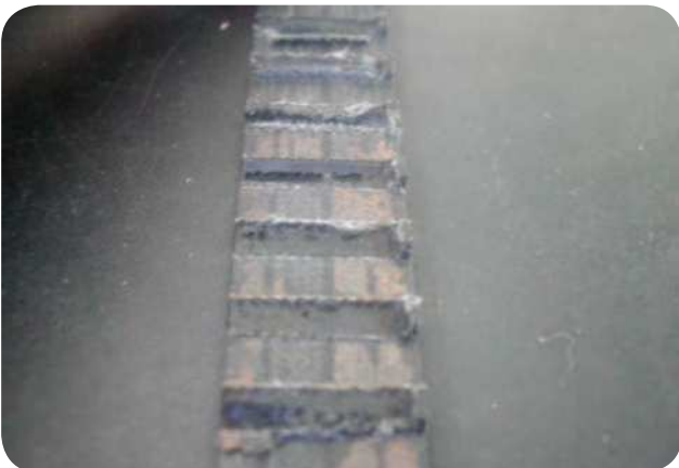
Belt is worn on one side, marks can be seen on the pulley.
