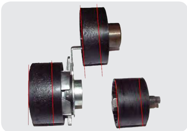
Belt ran on one side of the pulley.
