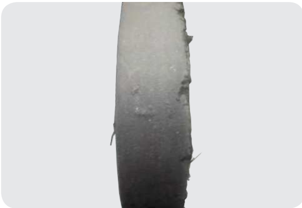
Belt is damaged on one of its flanges.
