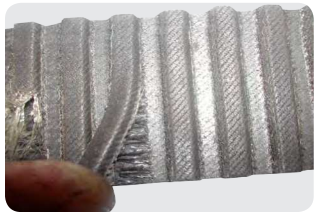
Belt teeth have been torn off.
