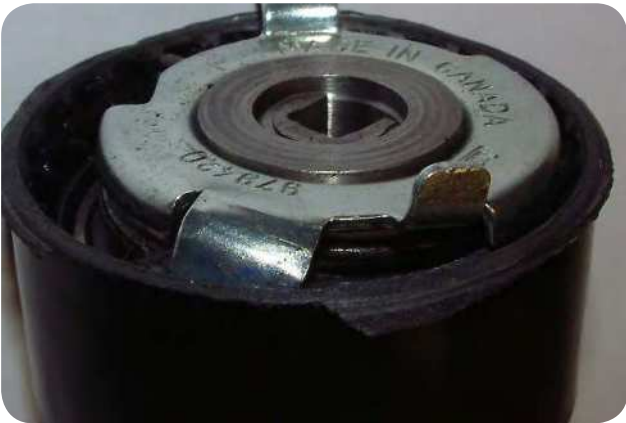
Hammering marks on the end stop or a cracked tensioner casting are clear signs of over tensioning.
