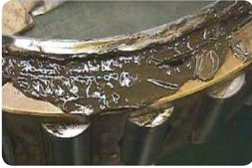
**Liquid contaminants reduce the lubricant viscosity**
