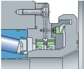
**Multiple seals in a bearing (housing) arrangement**
