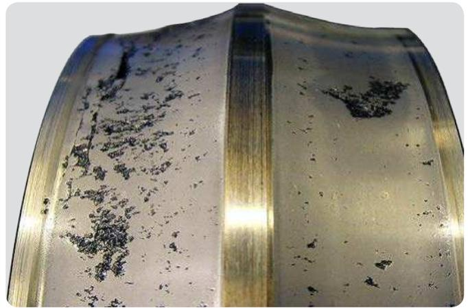
**Spherical roller bearing inner ring**
