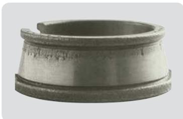
**Rolling surfaces are spalled due to material fatigue**
