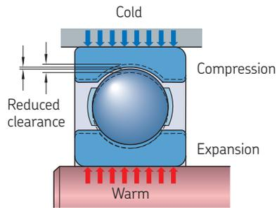
**Large temperature difference between the shaft and housing**
