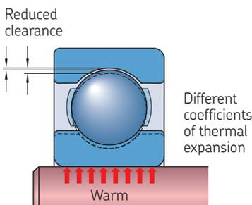
Shaft (and housing) material expands more than bearing steel
