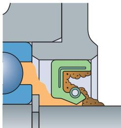
Seals oriented in the wrong direction and not allowing grease purge
