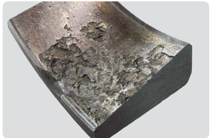
**Tapered roller bearing outer ring**
