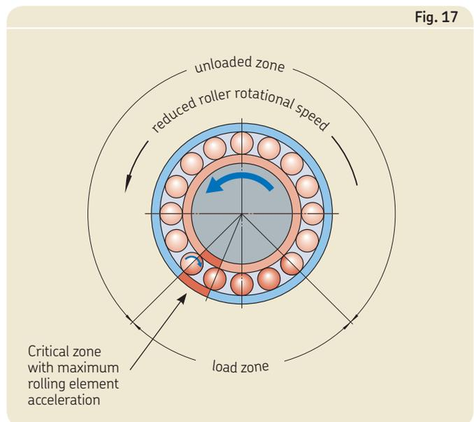
Smearing due to gyroscopic effects also occurs in ball bearings. In these cases, the balls change their contact angle when they are outside the load zone but are forced back (with slip) to their correct contact angle as they enter the load zone.
