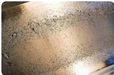
**Rolling surfaces are spalled due to surface initiated fatigue**
