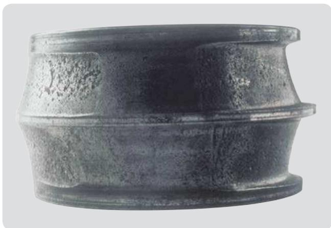
**Spherical roller bearing inner ring**
