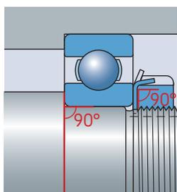
**Shaft and/or housing shoulders are out-of-square with the bearing seat**
