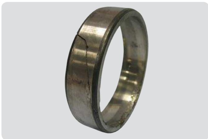
**Self-aligning ball bearing outer ring**
