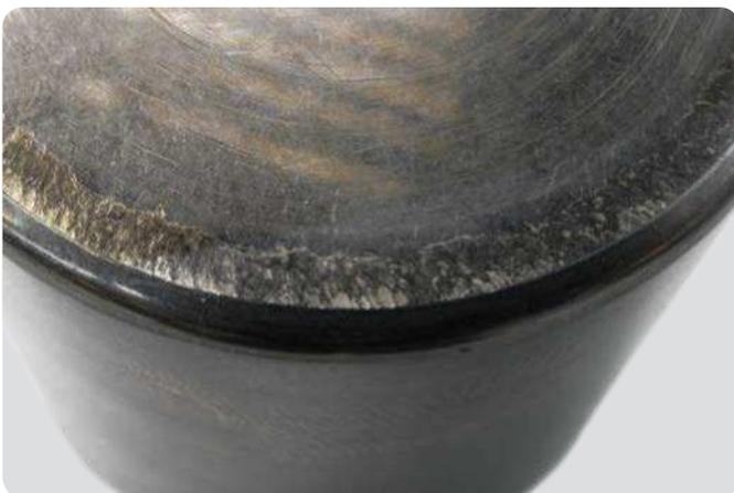
**Tapered roller bearing – roller**
