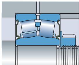
**Lock washer tabs are bent, fouling the cage or bearing seals**
