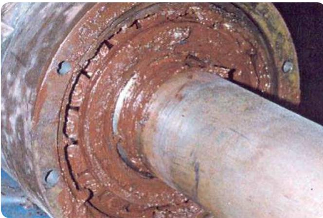
**Tapered roller bearing in a pump unit**
