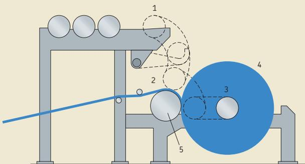
The reel drum is driven by the variable speed electric motor
