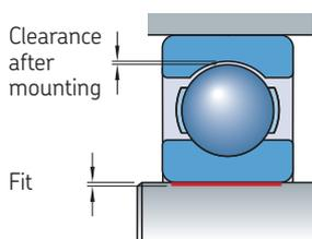
**Excessive shaft interference fit or oversized shaft seat diameter**
