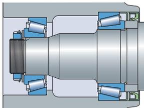
**Bearing adjustment results in excessive preload**
