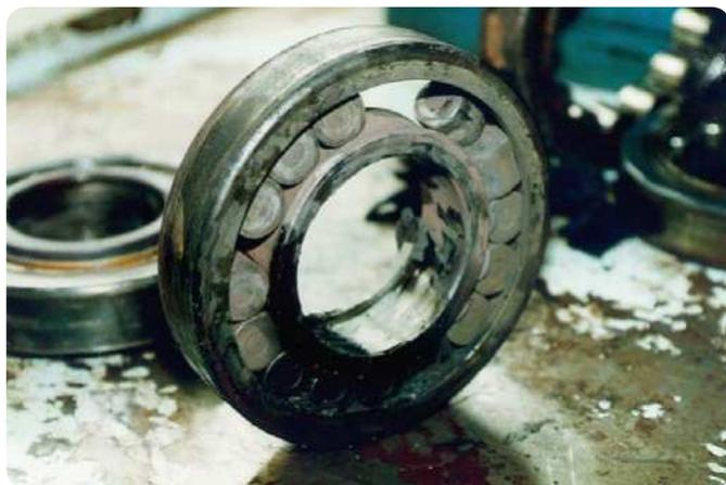
**Cylindrical roller bearing – inner ring, outer ring and rollers**
