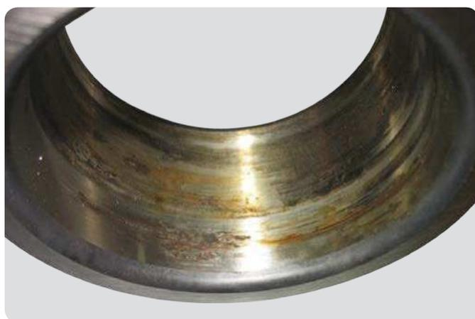
*Tapered roller bearing inner ring*
