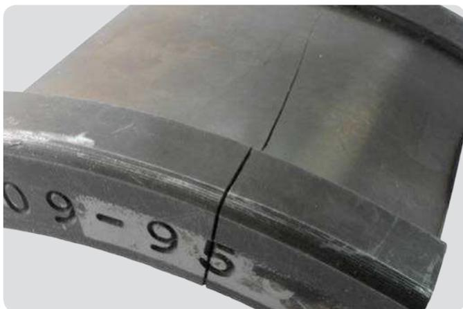
**Tapered roller bearing inner ring**
