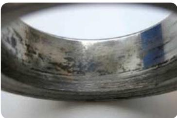
**Inner ring creeps (turns) on the shaft seat**
