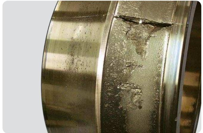
**Spherical roller bearing inner ring**
