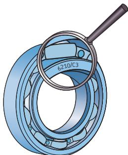
**Too large radial or axial internal clearance in a bearing**
