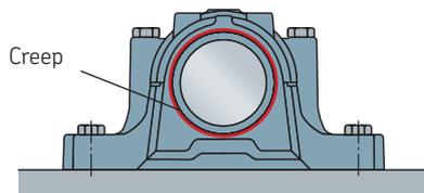
**Outer ring creeps (turns) in the housing seat**
