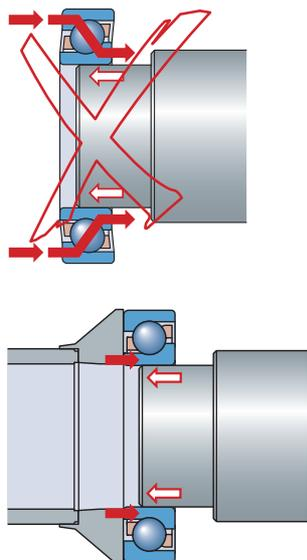
**Rolling surfaces are dented from impact or shock loads (incorrect mounting method)**
