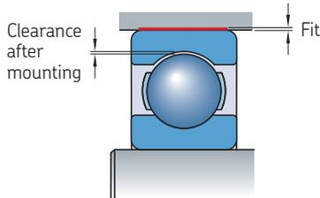
**Excessive housing interference fit or undersized housing seat diameter**
