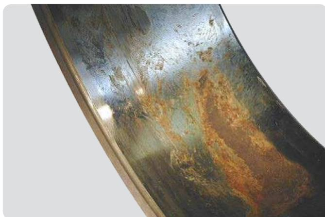
*Cylindrical roller bearing inner ring*
