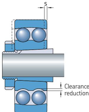
**Excessive drive-up on a tapered seat**
