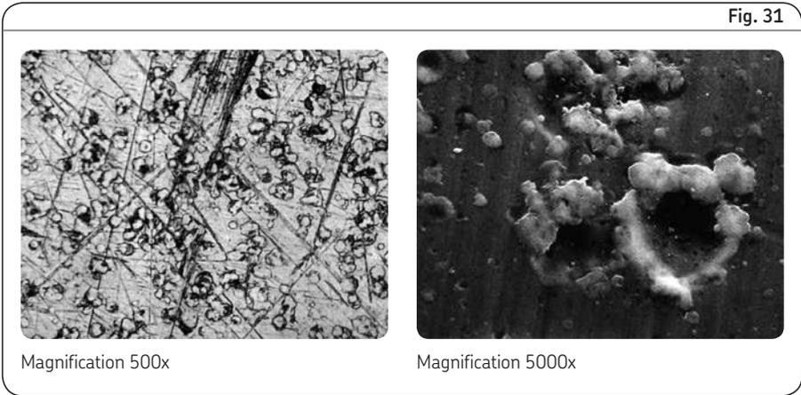
*Craters from current leakage erosion*
