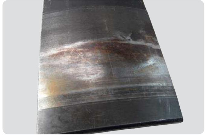
**Tapered roller bearing outer ring (phosphated)**
