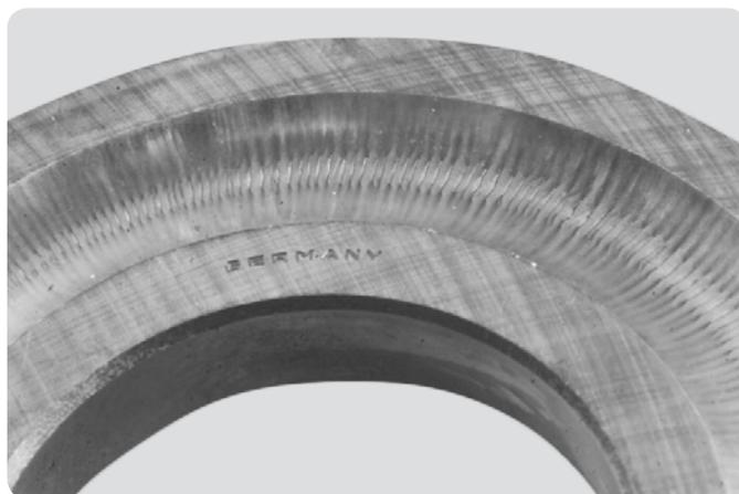
**Thrust ball bearing shaft washer**
