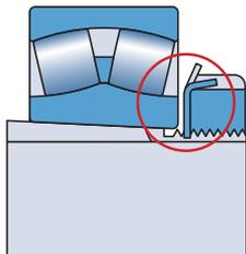
**The bearing lock nut is loose on the shaft or adapter sleeve**
