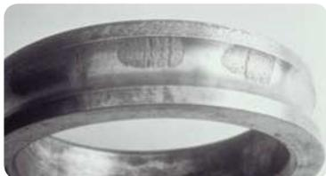
**Rolling surfaces are spalled, initiated from surface damage**
