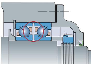
**The bearing is not clamped securely against mating components**
