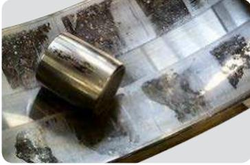
**Etching of rolling surfaces from chemical/liquid contaminants (water, acids, gasses, or other corrosives)**
