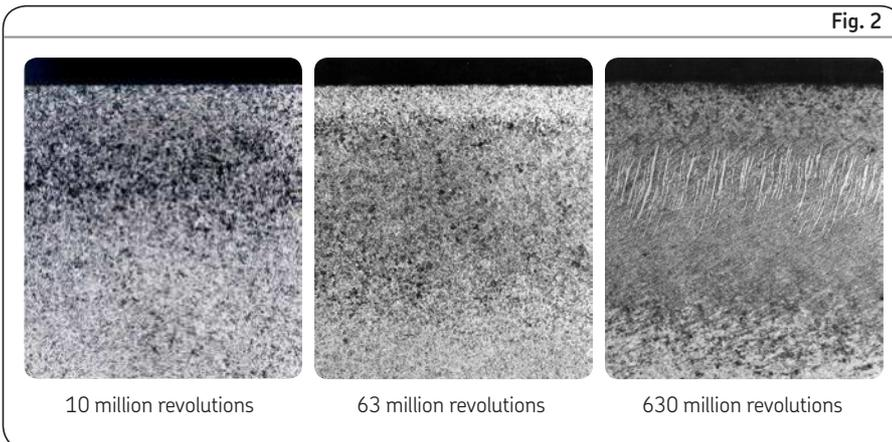
Crack development beneath the raceway surface (~ 0,3 mm)
