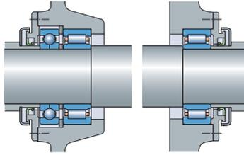
**The wrong bearing is (radially) located**
