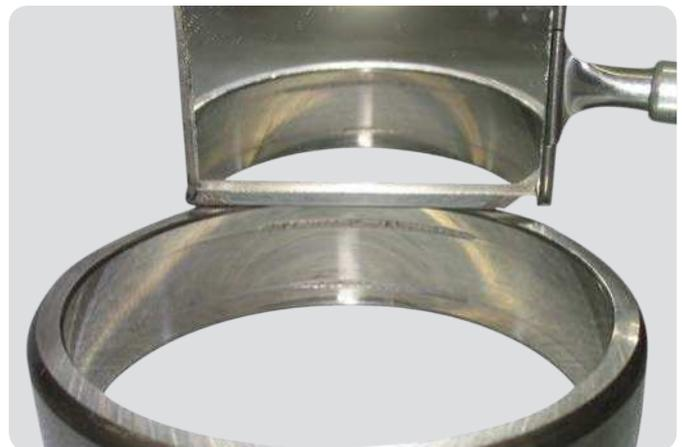
**Self-aligning ball bearing outer ring**
