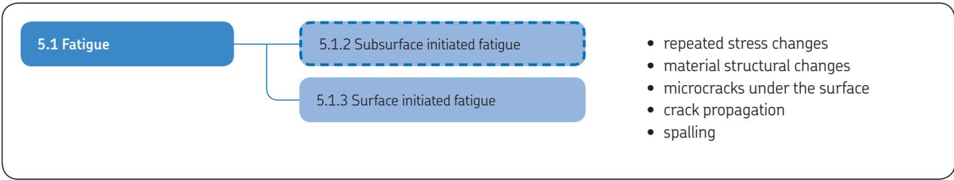
In a rotating bearing, cyclic stress changes occur beneath the contact surfaces of the raceways and rolling elements.
