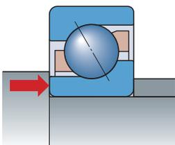
**Bearing installed backwards causing unloading of angular contact ball bearings**
