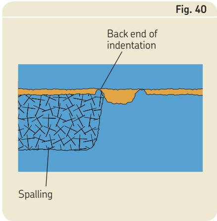
Spalling starting at the back end of an indentation
