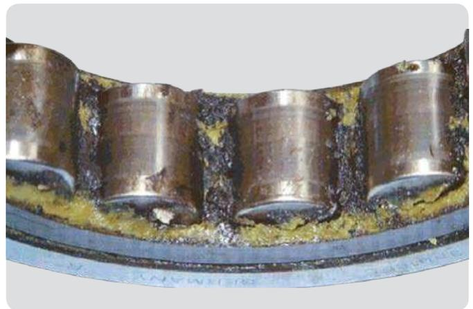
**Cylindrical roller bearing outer ring with cage, rollers and grease**
