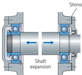
**Bearings are cross-located and the shaft can no longer expand**
