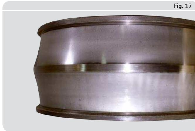
*Inner ring: Abrasive wear on the raceways*
