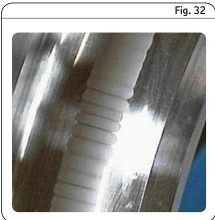
*Changes in material hardness resulting from current leakage*
