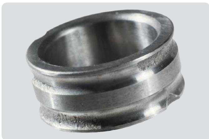
**Double row angular contact ball bearing inner ring**
