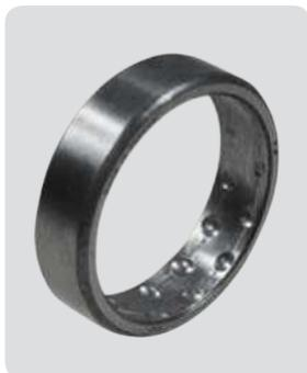
**Rolling surfaces are false-brinelled due to vibration**
