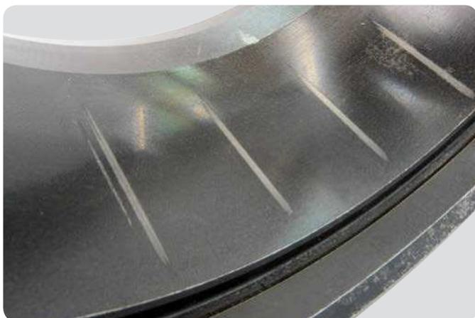
**Double row tapered roller bearing outer ring**
