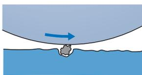
**Solid contaminants enter the bearing and dent the rolling surfaces**
