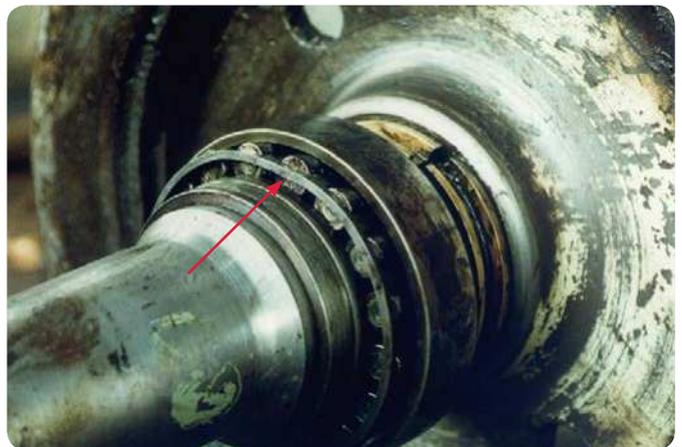
**Tapered roller bearing mounted on a railway wheel set**
