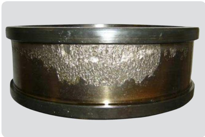
**Cylindrical roller bearing inner ring**
