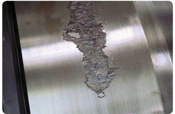
**Spherical roller bearing inner ring**
