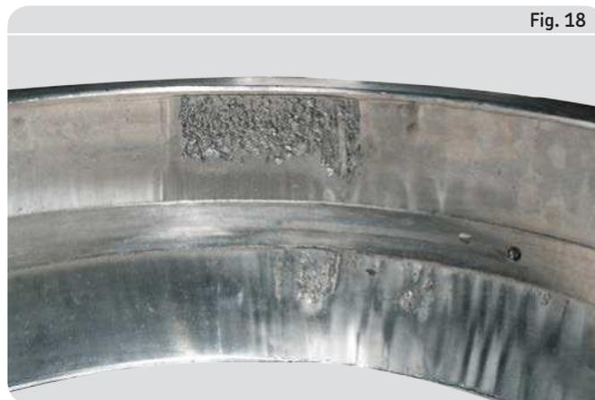
*Outer ring: Load zone spalls and vibration marks on the raceways, at the bottom of the ring*
