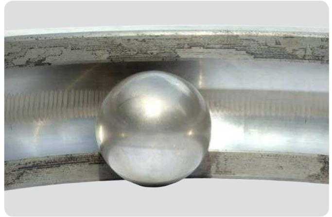
**Deep groove ball bearing outer ring and ball**
