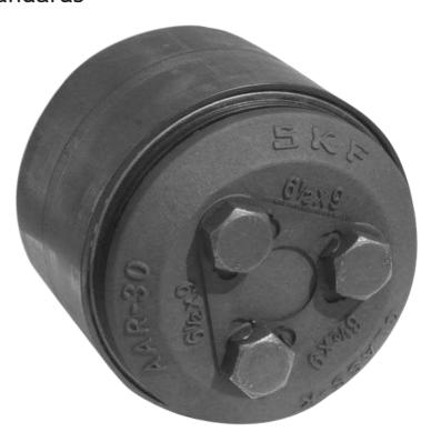
Tapered roller bearing units (TBUs) consist of two inner rings with a tapered roller and polymer cage assembly, a common outer ring, a central spacer, two sealing systems and a grease fill.
