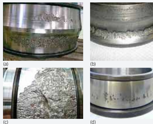
Fig. 3: Some typical examples of premature bearing failure from (a) paper machines, (b) compressors, (c) low-speed and (d) high-speed stages of a wind turbine gearbox.
