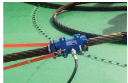
Newly installed wire rope lubricator on wire rope previously lubricated manually. Note: Even, clean penetrating distribution vs. uneven, messy coverage from previous method.
