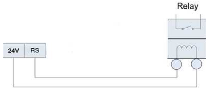
Figure 16 Connecting a relay to the Status, RS, relay driver output
