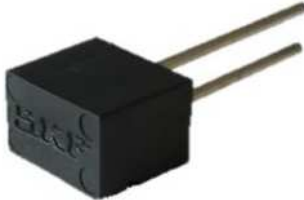
Figure 9 120-ohm resistor for RS485, bus termination
