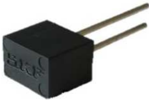
Figure 5 120-ohm resistor for RS-485, bus termination
