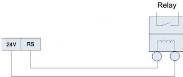
Figure 18 Connecting a relay to the Status, RS, relay driver output
