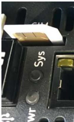
Figure 8 SIM card orientation
