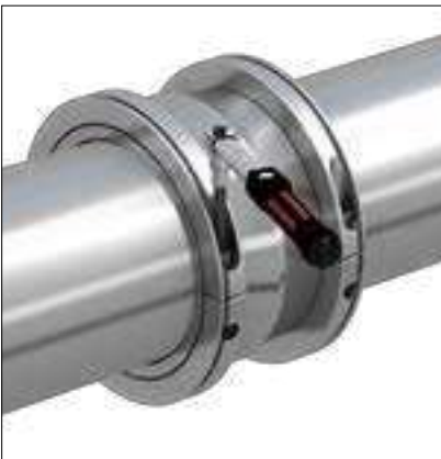
Figure 6. Inner ring and clamp rings on shaft. Note the gap between the rings
