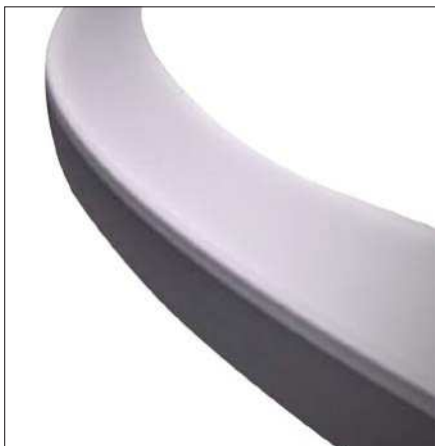
Kinetically sprayed zinc on a large-size SKF ring
