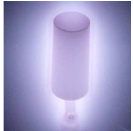
SKF rolling element surrounded by plasma in a vacuum chamber
