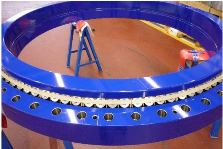
Test coating on an SKF large size bearing
