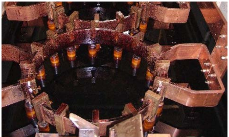
Sophisticated hard chromium anode frames at SKF
