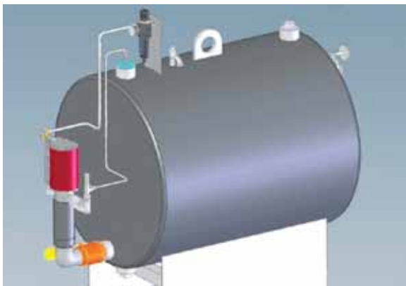
Fig. 26 Bulk Oil Storage Tank (BST)
