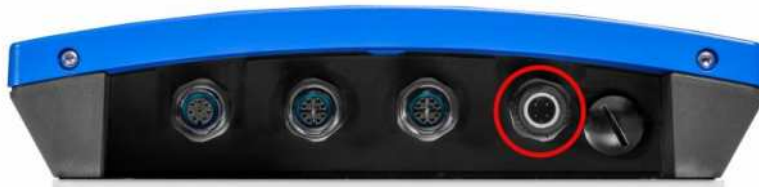
Figure 33 Incoming power supply connection
