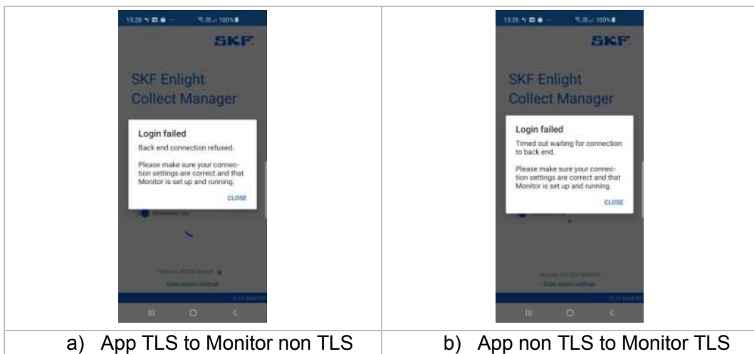
Figure 59 A mismatch of TLS settings causes connection errors
