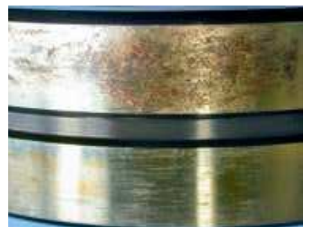
Figure 6. Fretting corrosion on the outer surface of a spherical roller bearing
