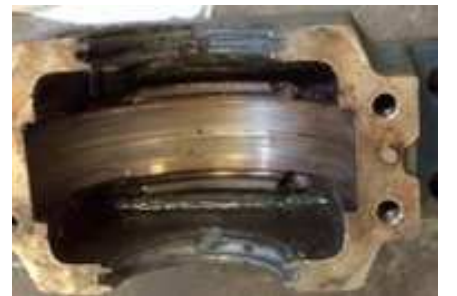
Figure 4. Worn housing bore due to outer ring rotation
