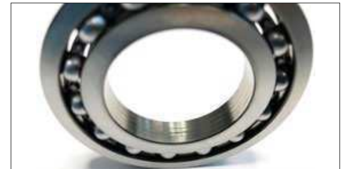
Figure 16. Circumferential scoring on inner bore
