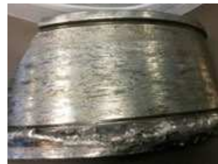
Figure 9. Excessive smearing in a tapered roller bearing (ring is fractured)
