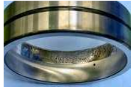
Figure 3. Excessive axial load on a spherical roller bearing, one raceway is damaged while the other is like new
