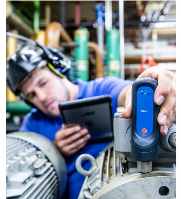
Figure 15. Example of QuickCollect system on site
