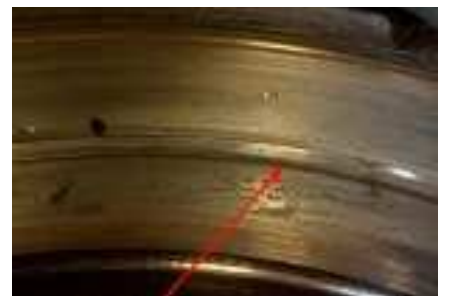
Figure 5. Closer view on a worn housing bore, the W33 lubrication groove pattern of the spherical roller bearing can be clearly seen
