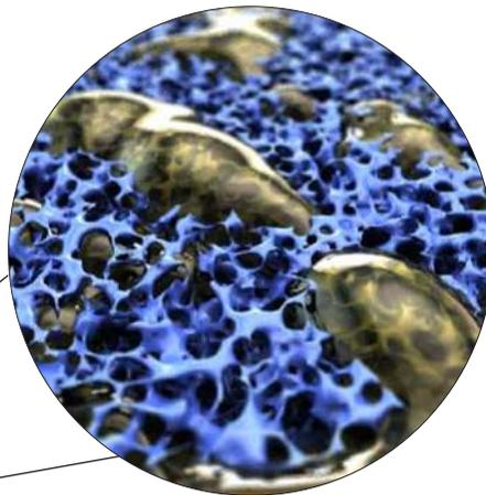
*Oil saturated polymer matrix having millions of micropores, releasing oil to the bearings raceways in operation.*
