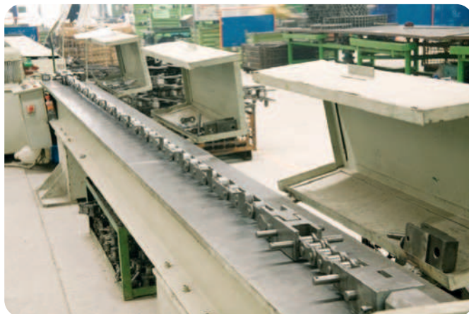
Pre-stressing after final assembly
