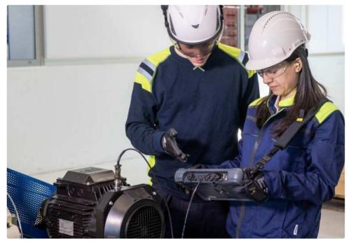
The Microlog dBX can be used as a standalone tool, taking measurements and analysing data from rotating machinery to determine machine health. It can also be connected to SKF monitoring software, such as the SKF @ptitude software suite, to handle analysis, on-premises and remote data storage, and download predefined measurement routes to the Microlog dBX.
