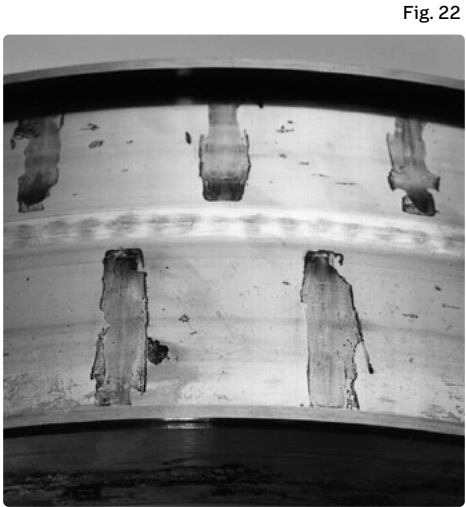
Initial patches of etching at rolling element spacings on the inner ring raceways of a spherical roller bearing
