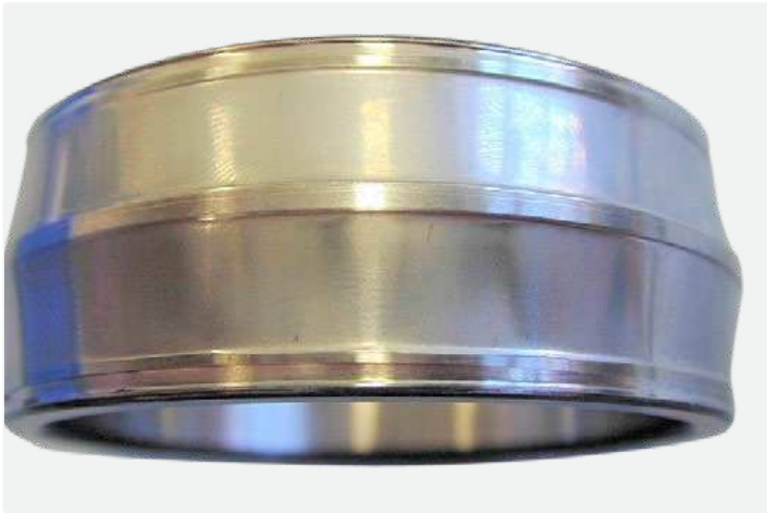
Spherical roller bearing inner ring Contamination and resulting inadequate lubrication leading to abrasive wear of the raceway tracks – slightly shiny
