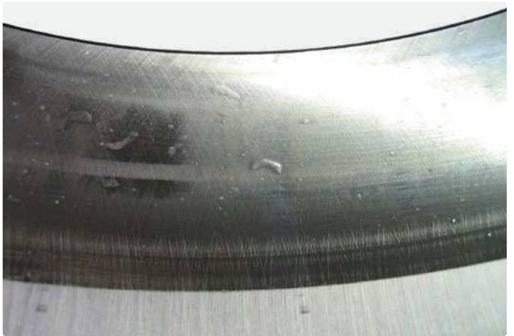
Spherical roller bearing outer ring Overrolling of swarf entered during mounting – lack of cleanliness
