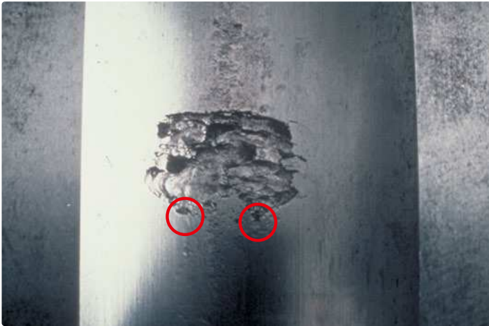
Deep groove ball bearing inner ring Overrolling of particles with sequential spalling starting at the back of the dents
