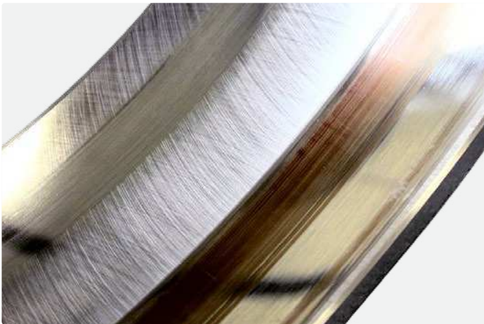
Spherical roller bearing outer ring Abrasive wear of the raceway tracks. The axially loaded one also partly discolored indicating inadequate lubrication and heat generation. The other raceway track shows a narrower load pattern with a matt appearance.
