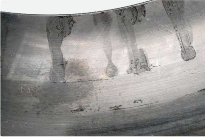
Spherical roller bearing outer ring Too high water content in lubricant, sets of etching marks at roller spacing at standstill
