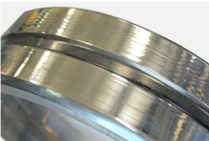
Spherical roller bearing outer ring Ring creep in the housing from inadequate housing fit for the load condition – polishing wear on the outside surface
