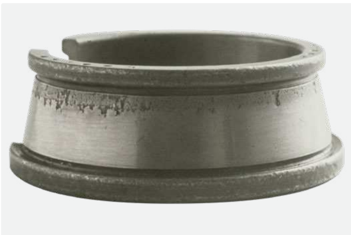
Tapered roller bearing inner ring Spalling on one side of the raceway only, resulting from misalignment and consequent edge loading, leading to higher stress and failure
