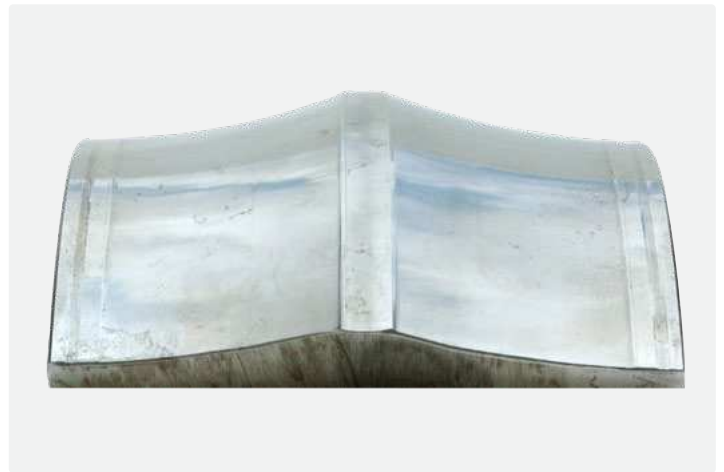
Spherical roller bearing inner ring Contamination by fine particles – abrasive wear of the raceway tracks – rather shiny. Due to cage pocket wear, a groove has been cut by the cages on either side.
