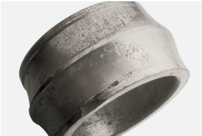
Spherical roller bearing inner ring Contamination and resulting inadequate lubrication leading to abrasive wear of the raceway tracks – one raceway track more damaged due to axial load
