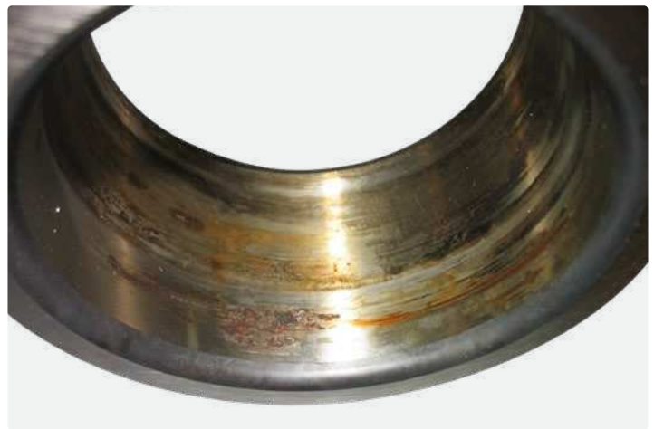
Tapered roller bearing inner ring Inappropriate shaft fit
