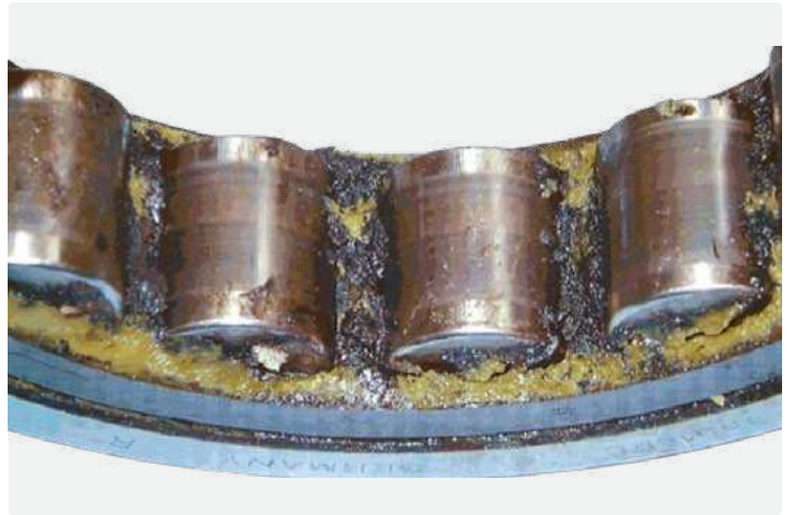
Cylindrical roller bearing outer ring with cage, rollers and grease Current leakage resulted in degradation of the grease (black) on the cage bars
