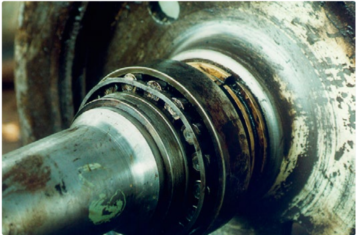
Tapered roller bearing mounted on a railway wheel set Cage was hit directly during mounting, resulting in permanent deformation (flattening)
