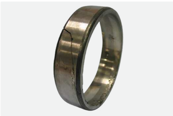
Self-aligning ball bearing outer ring Fracture resulting from excessive misalignment and balls running over the raceway edge
