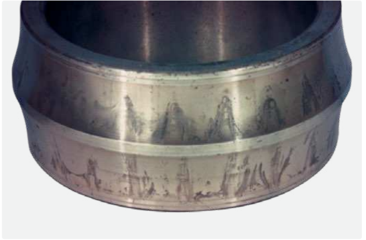
Spherical roller bearing inner ring Lubricant contaminated by water, etching marks at roller spacing at standstill
