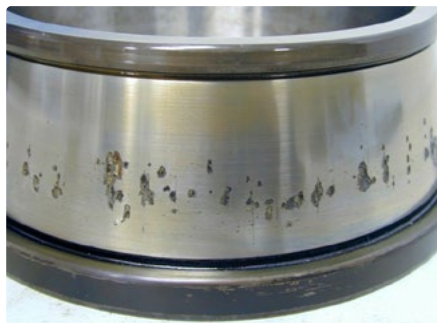
Premature subsurface initiated fatigue - Calotte spalling of steel balls caused by hydrogen induced cracking from \text{CO}_2 and condensing water (left), general spalling due to stress overload (center), white etched crack (right)
