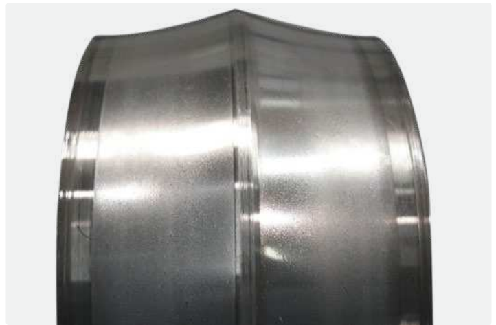
Spherical roller bearing inner ring Many small dents resulting from overrolling of small hard particles – inadequate sealing arrangement
