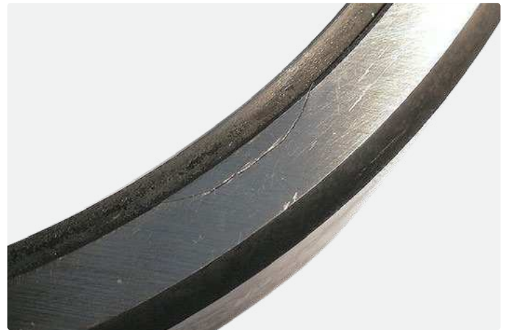
Deep groove ball bearing outer ring side face Fracture at seal anchorage groove due to impact when mounting the bearing
