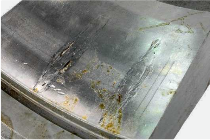
Double row tapered roller bearing outer ring Overload impact and misalignment at standstill, resulting in deformation and subsequent spalling at roller spacing
