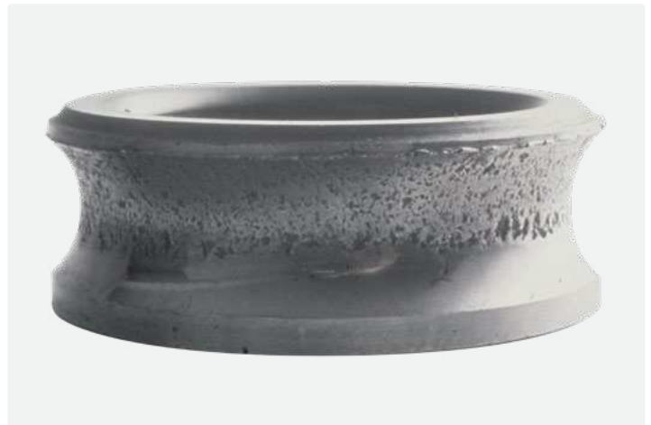
Deep groove ball bearing inner ring Excessive axial load, resulting in too thin lubricant film and surface distress
