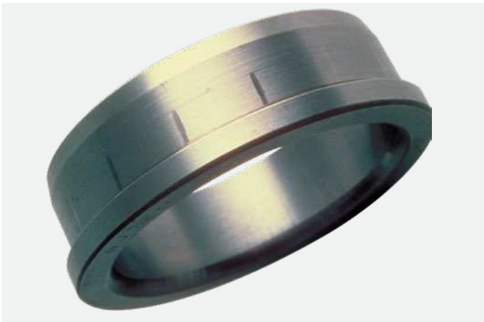
Cylindrical roller bearing inner ring During the assembly procedure, inner and outer rings were not aligned properly. Axial marks at roller spacing.
