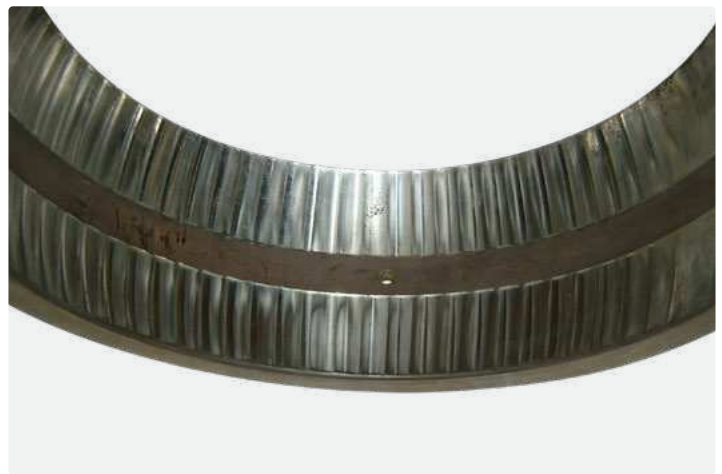
Spherical roller bearing outer ring Exposure to excessive vibrations at standstill, sets of false brinelling marks at roller spacing
