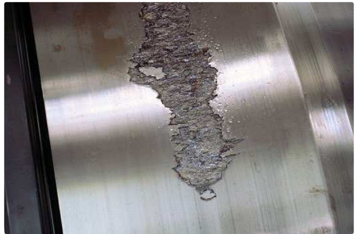
Spherical roller bearing inner ring Material fatigue
