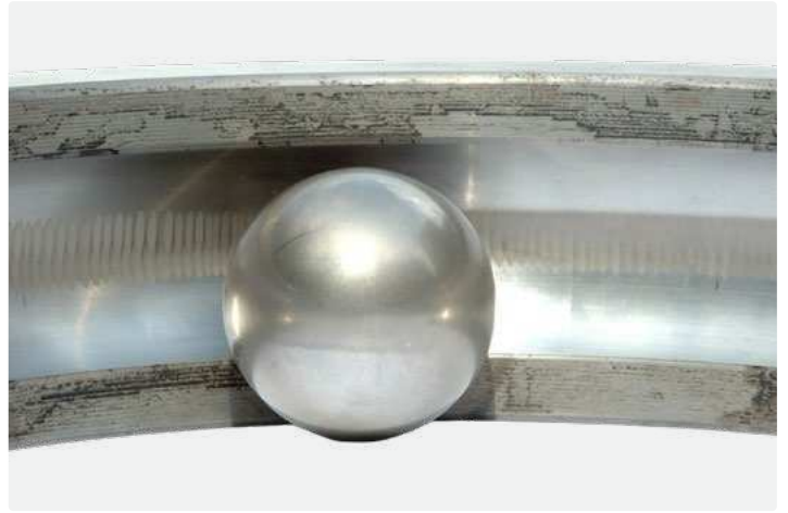
Deep groove ball bearing outer ring and ball Fluting in the outer ring and dull ball surface
