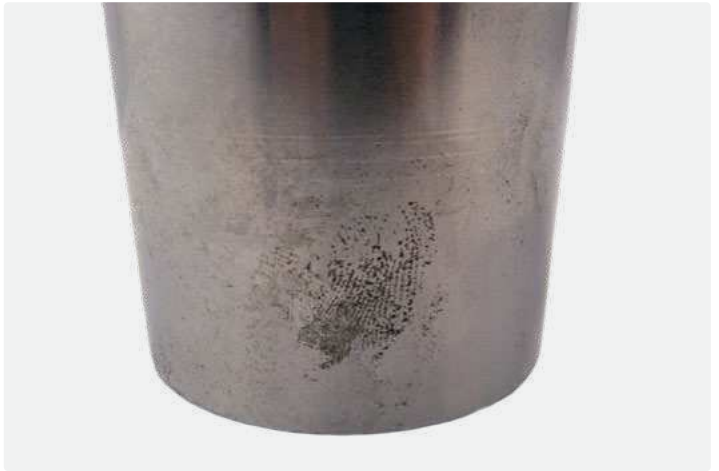
Tapered roller bearing – roller Rusty surface on raceway resulting from finger perspiration
