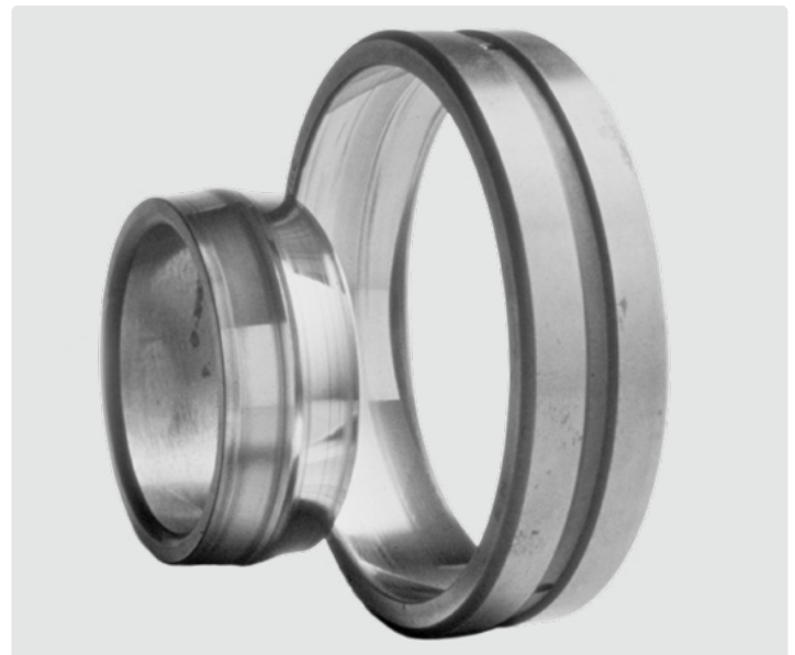
Polishing wear (mirror-like raceway surfaces) on the inner and outer rings of a spherical roller bearing
