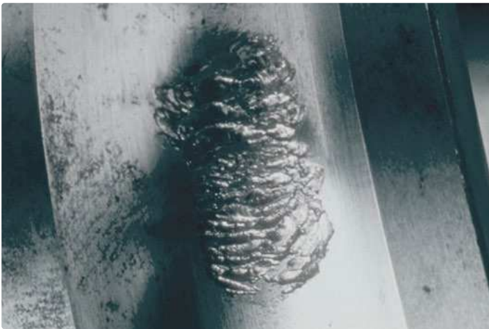
Deep groove ball bearing inner ring Material fatigue
