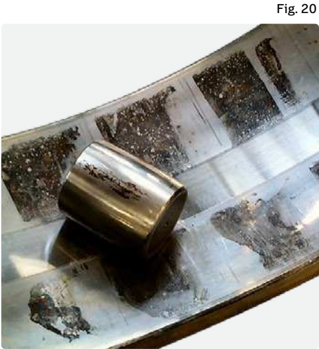
Corrosion on the outer ring raceways and roller of a spherical roller bearing
