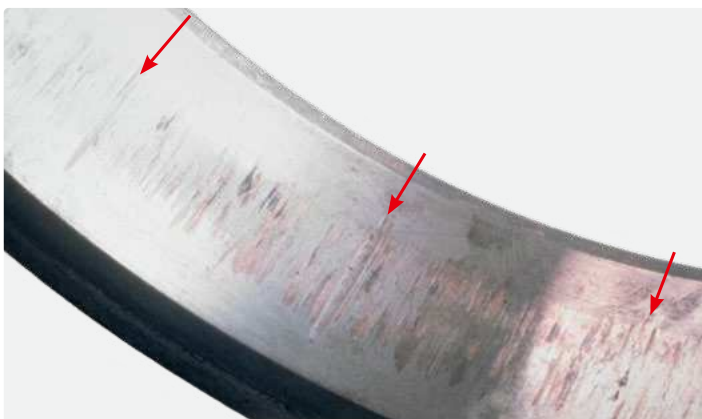
False brinelling on the outer ring raceway of a cylindrical roller bearing
