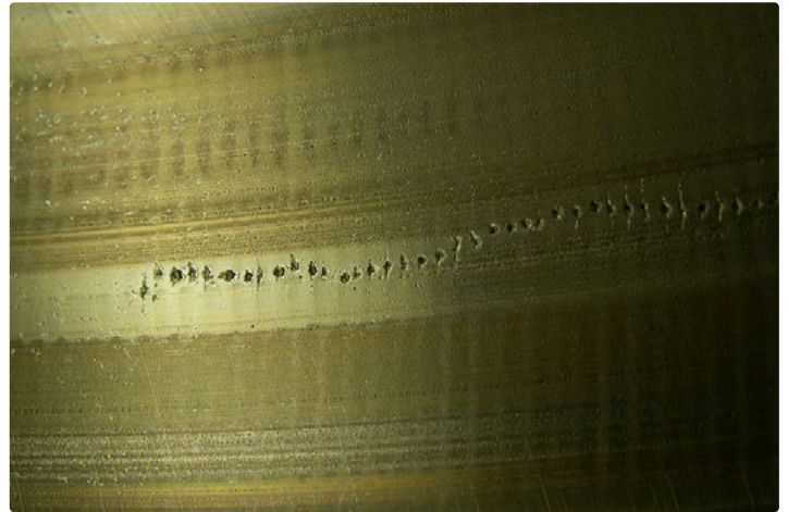
Spherical roller bearing – roller Enlarged view of craters in a bead-like formation
