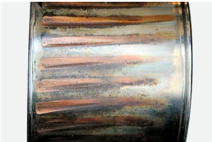
CARB toroidal roller bearing inner ring Exposure to vibrations at standstill with small oscillatory movements, false brinelling marks at roller spacing
