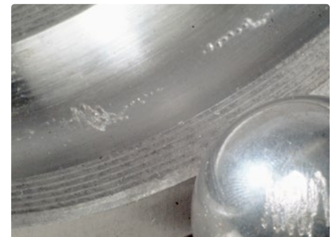
Excessive current erosion on the outer ring raceway and ball of a deep groove ball bearing
