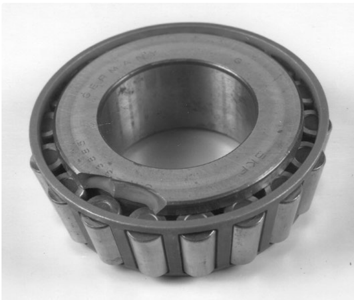
Fracture on the large shoulder of a tapered roller bearing inner ring resulting from rough treatment
