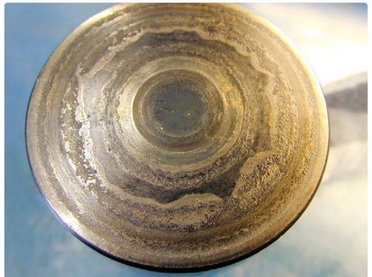
Smearing on a roller thrust face of a spherical roller thrust bearing
