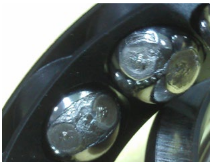
Premature subsurface initiated fatigue - Calotte spalling of steel balls caused by hydrogen induced cracking from \text{CO}_2 and condensing water (left), general spalling due to stress overload (center), white etched crack (right)
