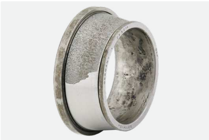
Tapered roller bearing inner ring Inadequate lubricant film, surface distress over a large area
