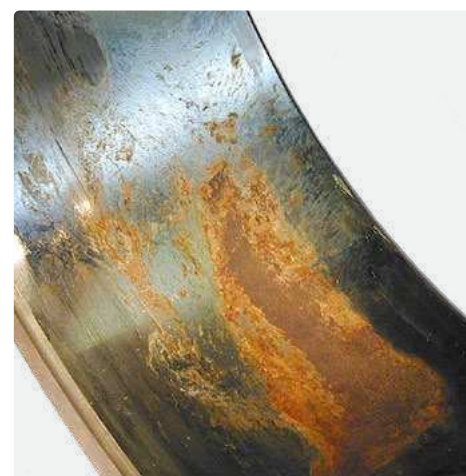
Fretting corrosion on an inner ring bore resulting from heavy load or inadequate shaft seat
