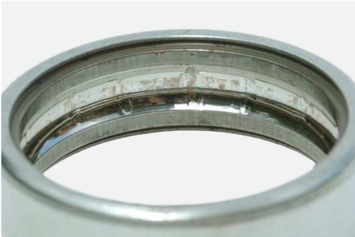
Deep groove ball bearing outer ring Plastic deformation at ball spacing from applying mounting force to the wrong ring
