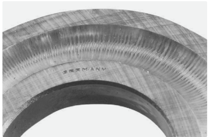
Thrust ball bearing shaft washer Exposure to vibrations at standstill, several sets of false brinelling marks at ball spacing
