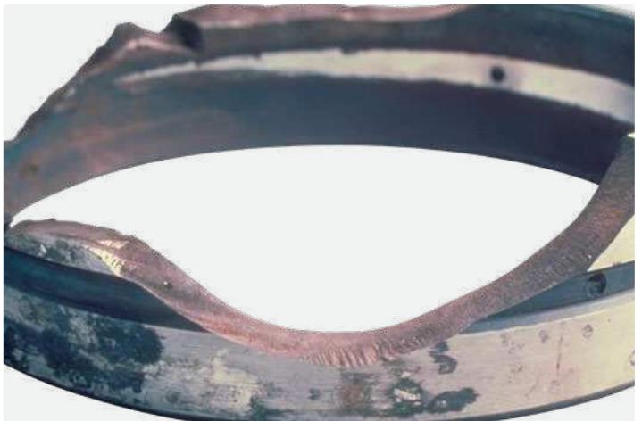
Spherical roller bearing outer ring Inadequate housing seat leading to fretting corrosion and finally fatigue fracture
