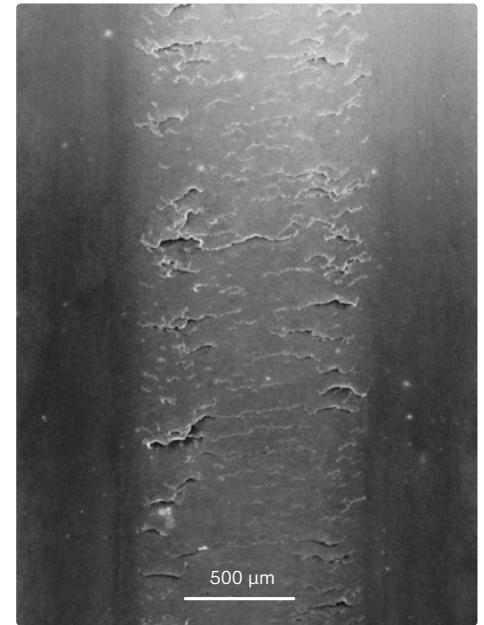
Initial spalling resulting from surface initiated fatigue on the inner ring raceway of a deep groove ball bearing
