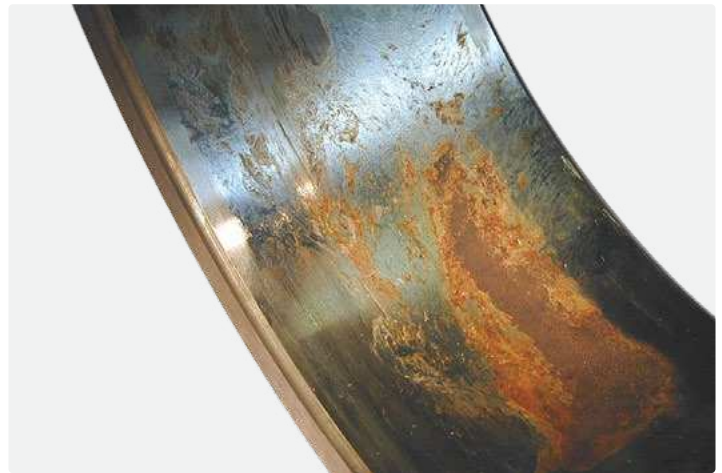
Cylindrical roller bearing inner ring Inappropriate shaft fit, uneven support
