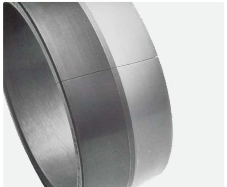
Fractured inner ring of a spherical roller bearing with a tapered bore resulting from excessive drive-up
