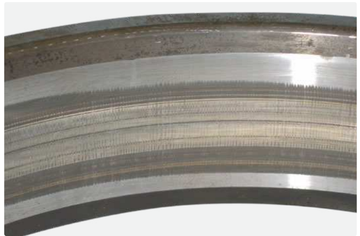
Cylindrical roller bearing outer ring Early stage of fluting
