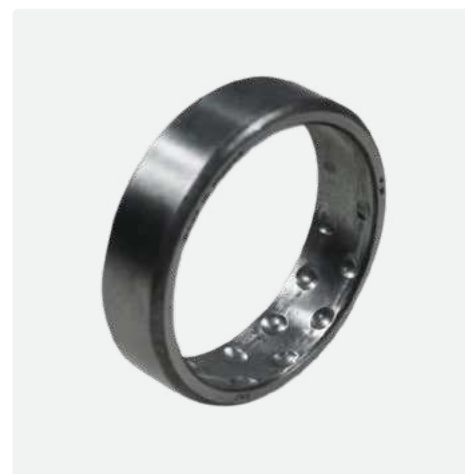
Severe false brinelling on the outer ring raceway of a self-aligning ball bearing
