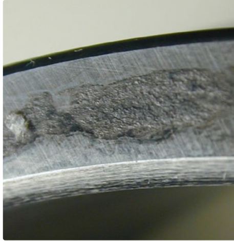
Outer ring: Fretting corrosion on the side face
