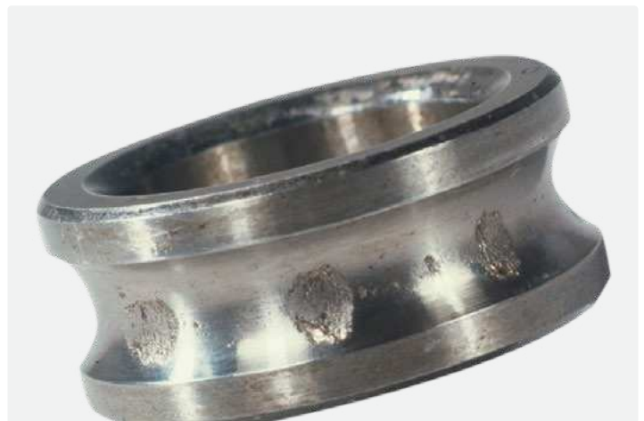
Deep groove ball bearing inner ring Impact during mounting, resulting in spalling at ball spacing
