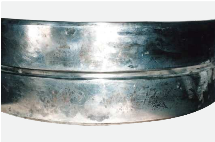
Outer ring: Heavy fretting corrosion in the load zone of the outside surface
