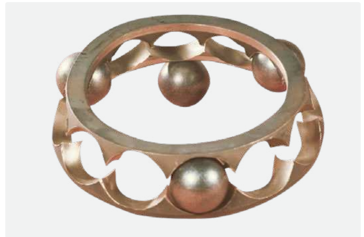
Angular contact ball bearing cage Abrasive wear of the cage pockets due to inadequate lubrication and vibration. Cage bars worn away.
