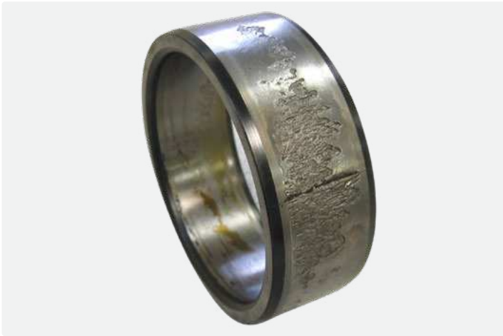
Cylindrical roller bearing inner ring Very heavy spalling – fatigue fracture as sequential damage
