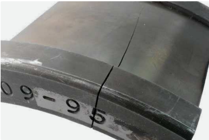
Tapered roller bearing inner ring The bearing was fitted to an oversized shaft
