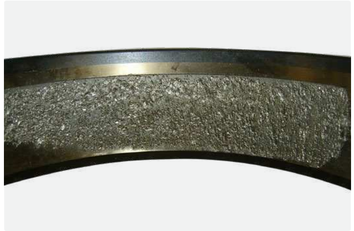
Cylindrical roller bearing outer ring Inadequate lubricant film, some misalignment, advanced surface distress
