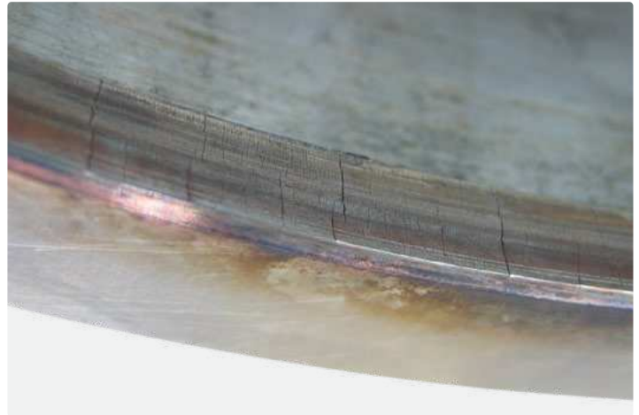
Cylindrical roller bearing outer ring Thermal cracks at shoulder-cage contact due to inadequate lubrication
