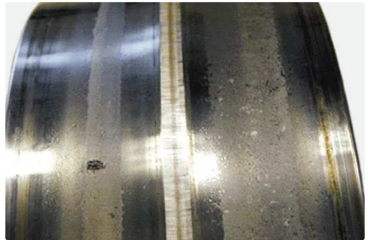
Spherical roller bearing inner ring Ingress of contaminants leading to inadequate lubrication, abrasive wear on the tracks and one incipient spall
