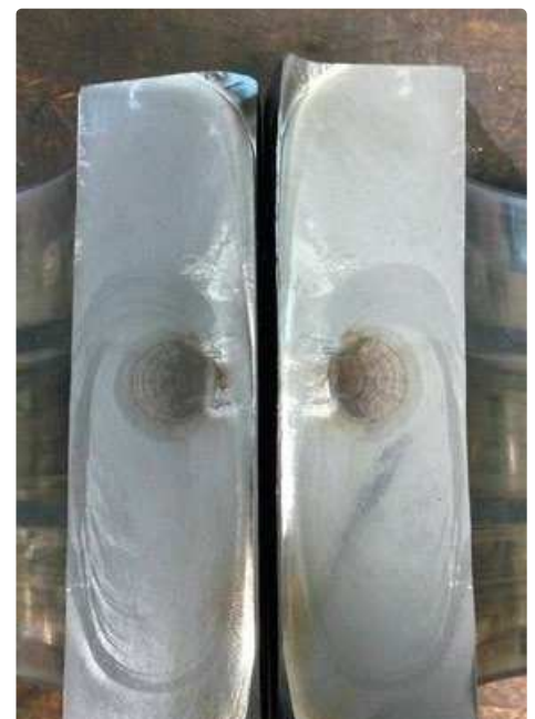
Fatigue fracture of cylindrical roller bearing outer ring
