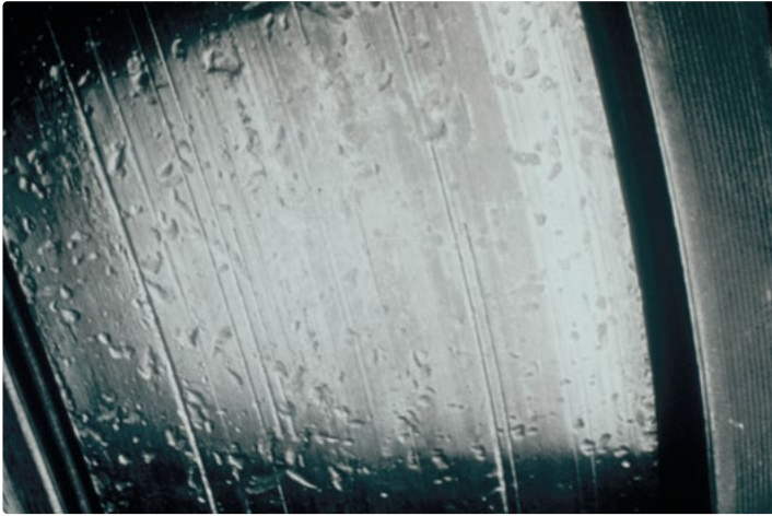
Tapered roller bearing inner ring Overrolling of big and hard particles that entered the bearing due to inadequate sealing arrangement
