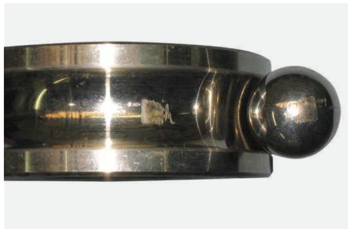
Deep groove ball bearing inner ring and ball Excessive current resulting in a number of craters in zig-zag formation on the ball and raceway
