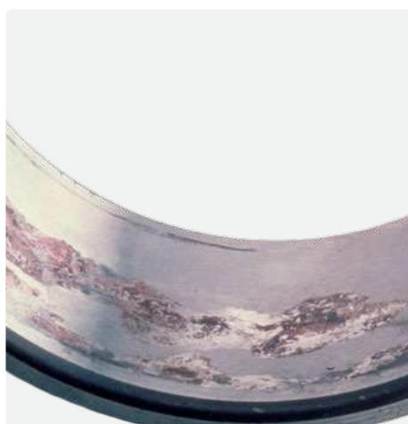
Fretting corrosion on an inner ring bore resulting from an inadequate shaft seat or shaft bending
