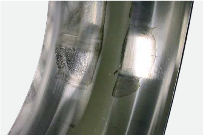
Spherical roller bearing outer ring Sealing arrangement failure, corrosion at standstill
