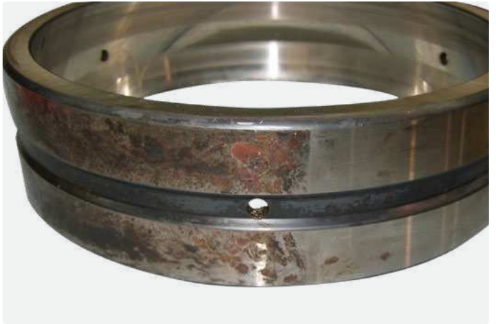
Spherical roller bearing outer ring Inadequately supported ring
