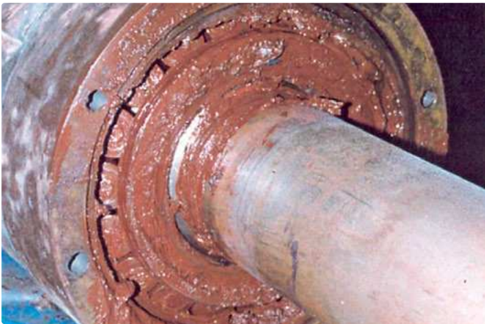
Tapered roller bearing in a pump unit Seal failure, bearing corrosion and reddish discoloured grease
