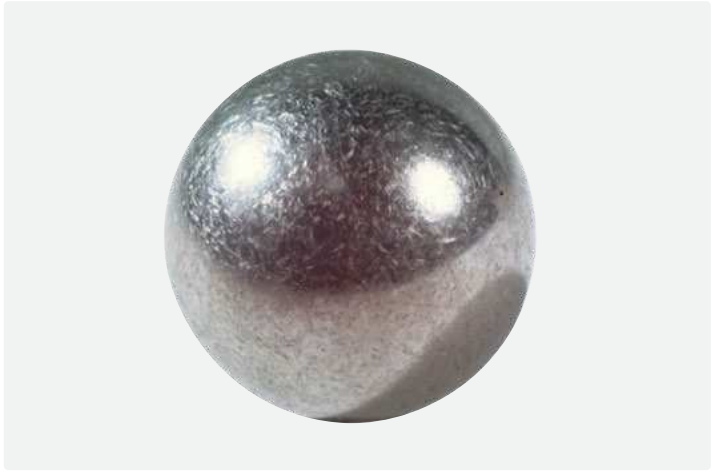
Deep groove ball bearing – ball Damage resulting from hard particles in very contaminated lubricant
