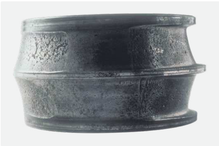
Spherical roller bearing inner ring Inner ring stationary – heavy abrasive wear – two wear zones: one with heavy wear; then creep of the inner ring with subsequent second wear zone
