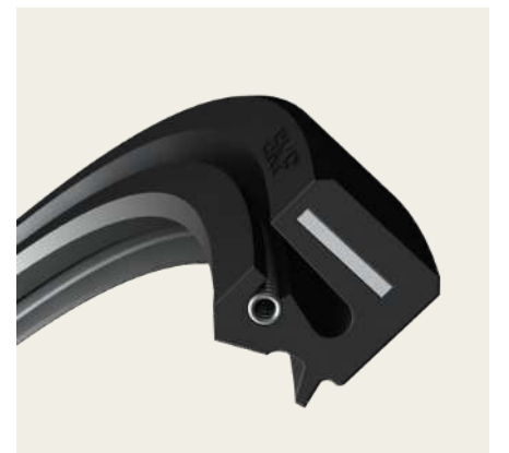
Rubber metal reinforced, self retaining seal with auxiliary lip
