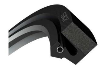
The TR/3 solid back and lip area provide a good flexibility, to compensate shaft misalignment and a maximum pressure of 0,5 bar. Furthermore, the spring embedding has been carefully studied to prevent its tilting during mounting.
